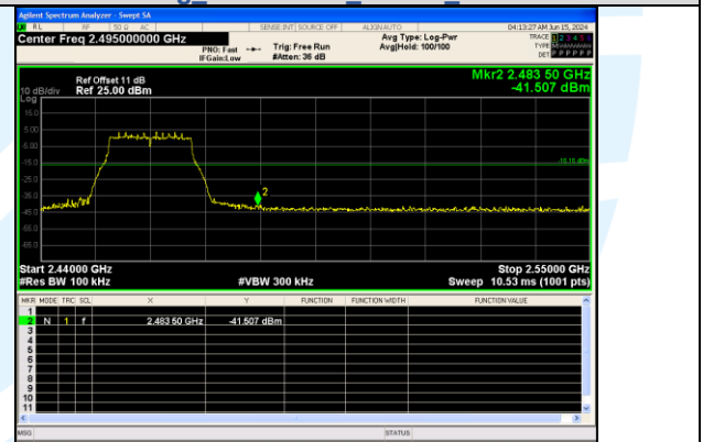
Out Of Band Emission IEEE 802.11g Channel 11 20MHz Antenna 0
