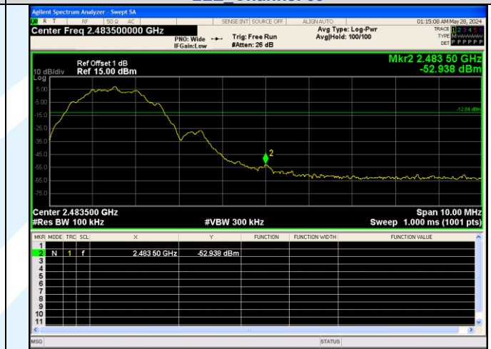
Out Of Band Emission 2LE Channel 39
