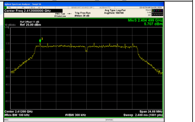
In-Band Reference Level IEEE 802.11g Channel 1 20MHz Antenna 0
