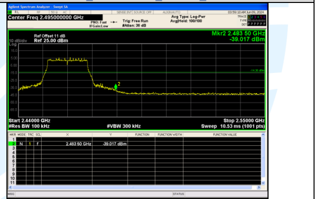
Out Of Band Emission IEEE 802.11n Channel 11 20MHz Antenna 0
