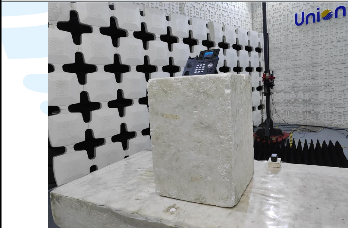
Radiated emission Test Setup (Above 1 GHz)
