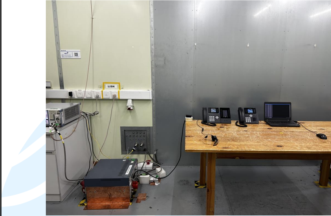
Conducted Emission Test Setup
