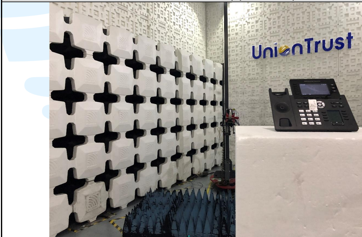
Radiated emission Test Setup (Above 1 GHz)
