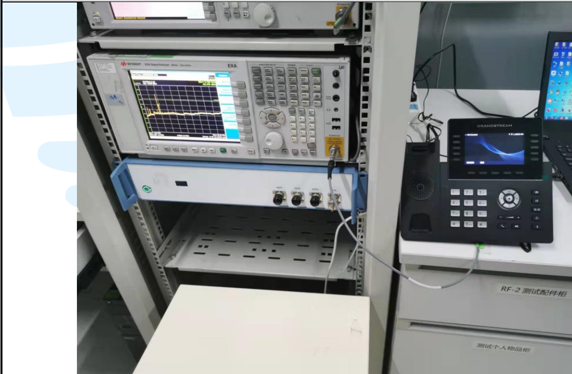
RF Conducted Test Setup
