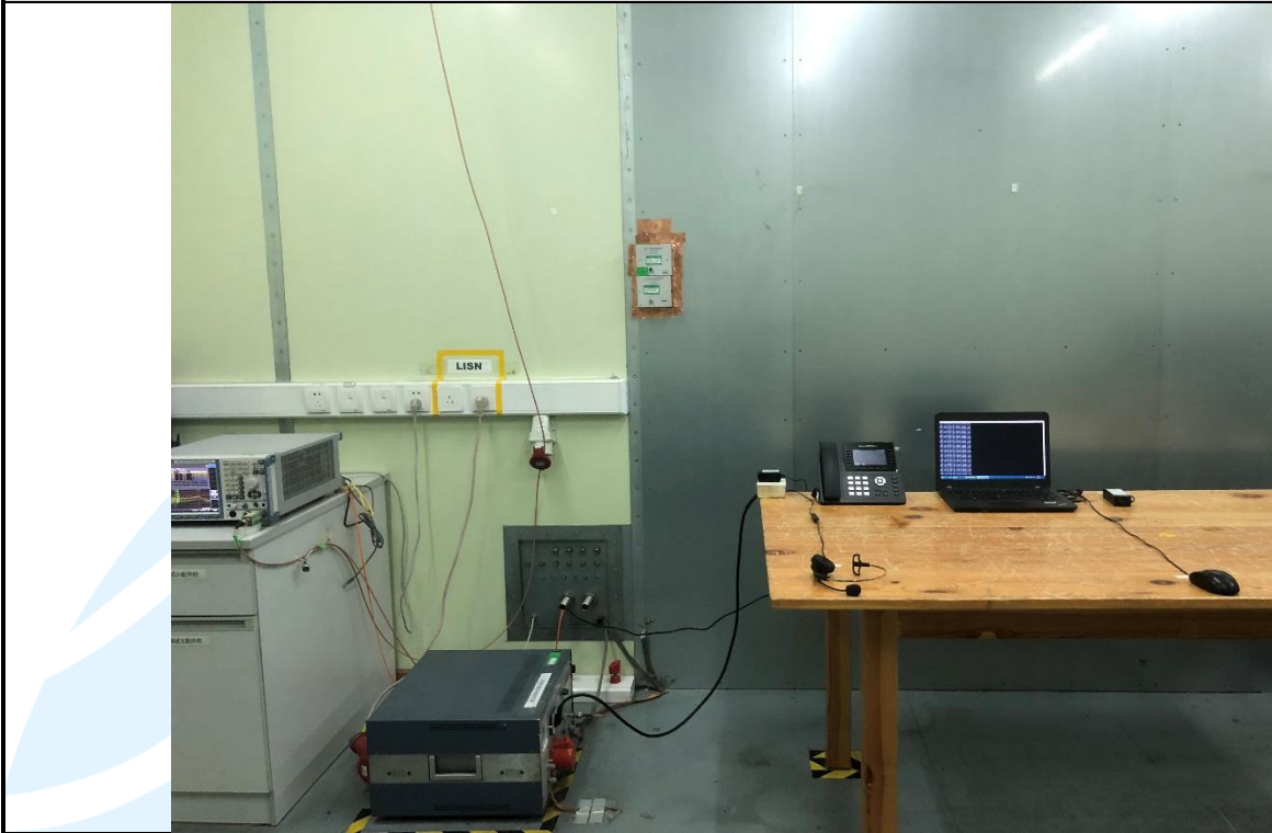
Conducted Emission Test Setup
