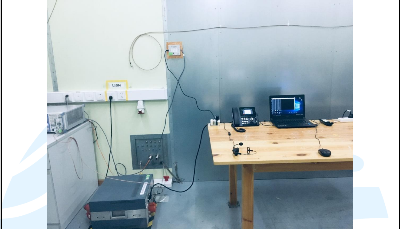
Conducted Emission Test Setup
