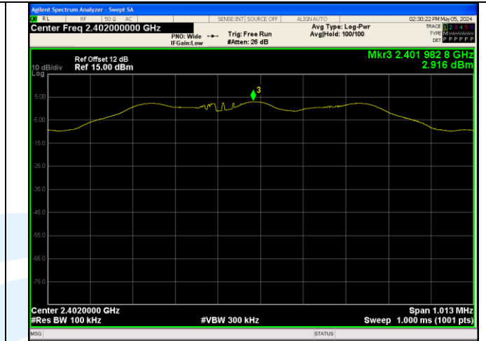
In-Band Reference Level LE Coded (S=8) Channel 0
