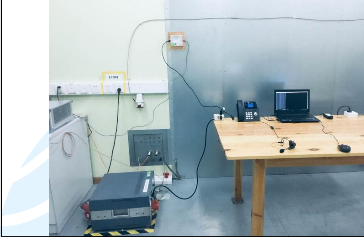
Conducted Emission Test Setup
