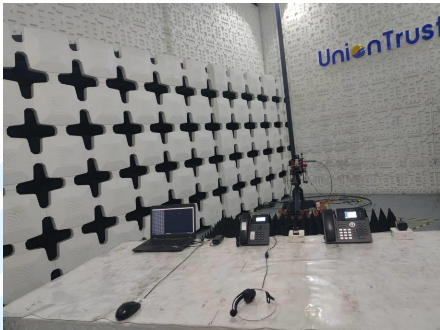
Radiated emission Test Setup-2 (Above 1 GHz)
