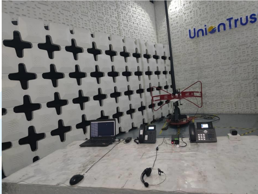
Radiated emission Test Setup-1 (30 MHz~1 GHz)
