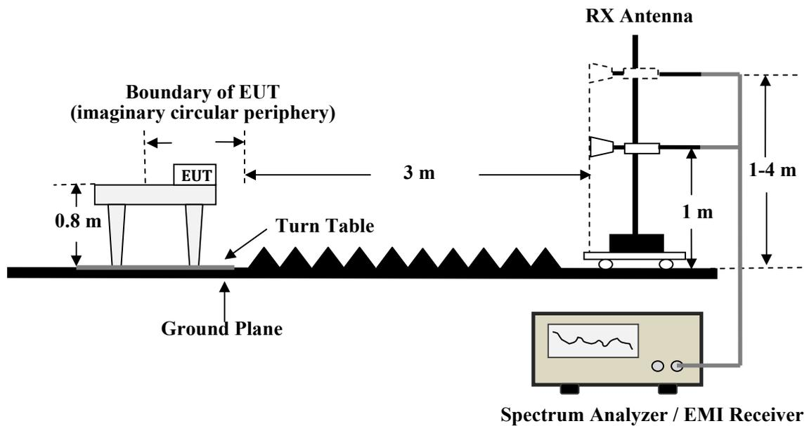
**Radiated Emissions Setup Configuration**
