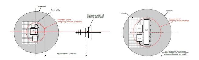
The radiated emission tests were performed in the 3 meters chamber test site, using the setup accordance with the ANSI C63.4-2014. The related limit was specified in FCC Part 15B.
