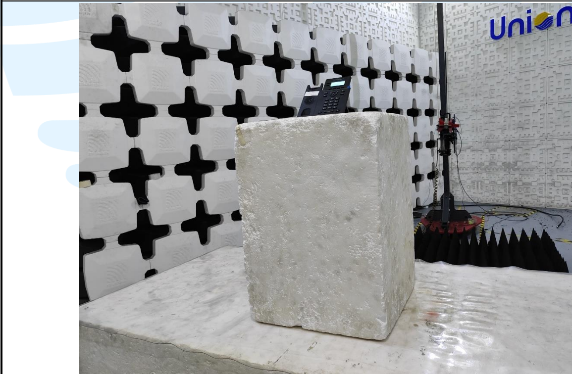
Radiated emission Test Setup (Above 1 GHz)
