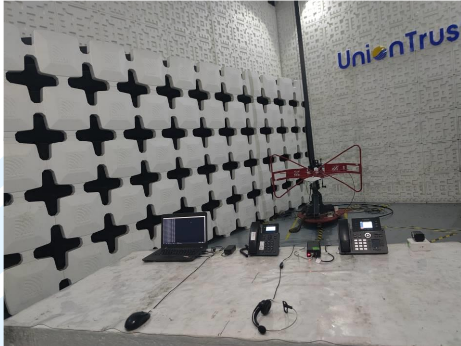
Radiated emission Test Setup-1 (30 MHz~1 GHz)
