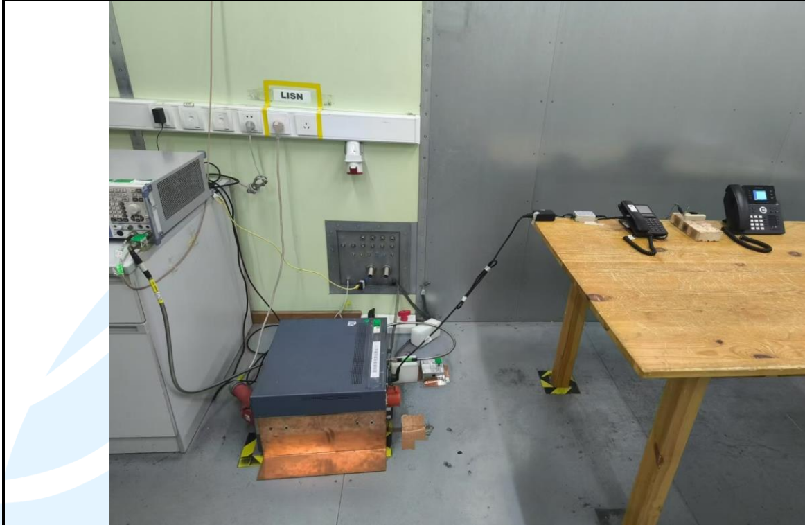
Conducted Emission Test Setup
