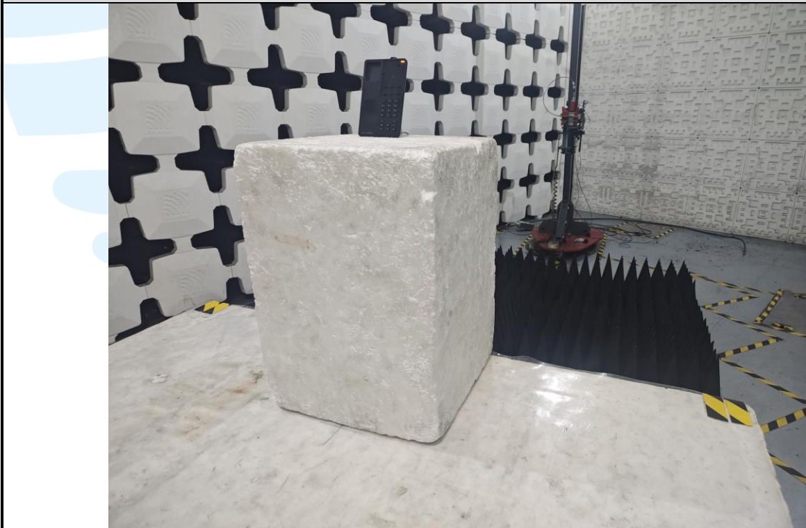
Radiated emission Test Setup (Above 1 GHz)
