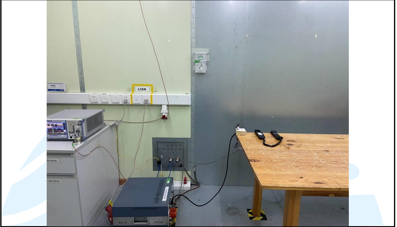
Conducted Emission Test Setup
