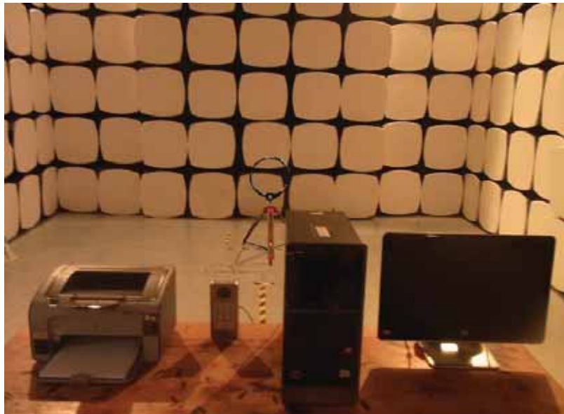
Radiated Emission Test Set-up(9KHz-30MHz)
