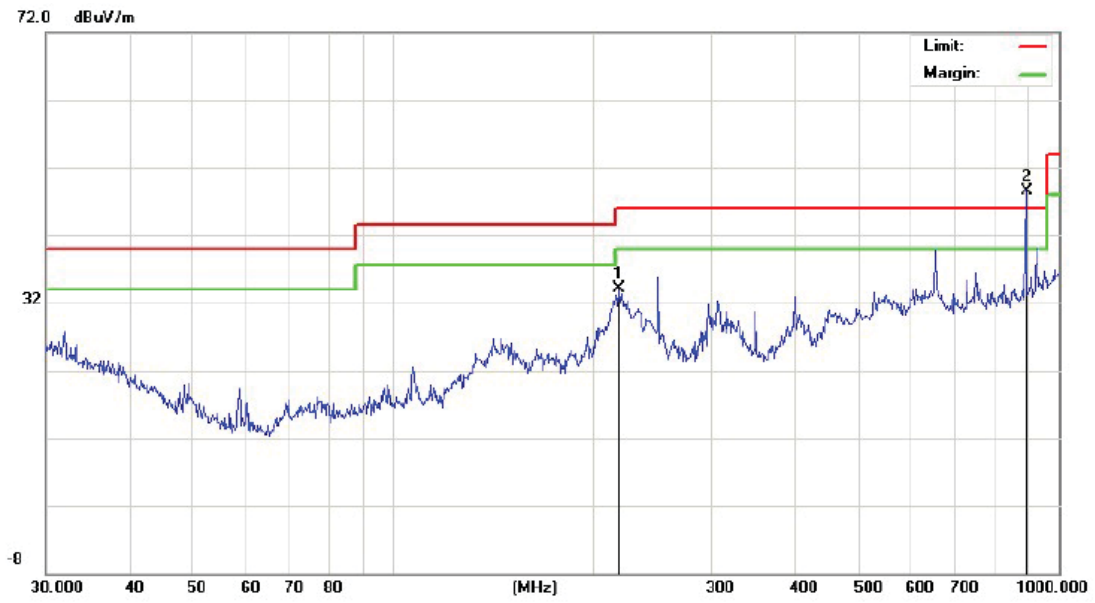
Horizontal: Radiated Emission Test Plot(30-1000MHz)
