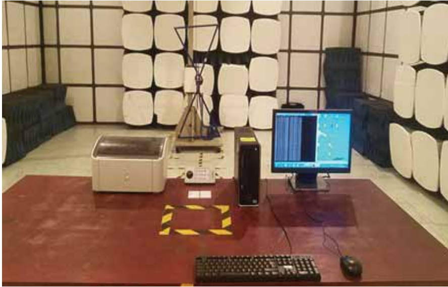
Radiated Emission Test Set-up(30-1000MHz)
