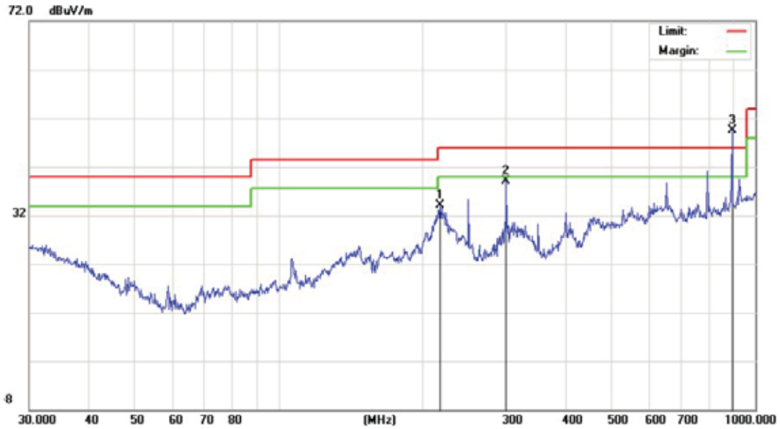
Horizontal: Radiated Emission Test Plot(30-1000MHz)
