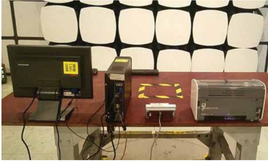
Radiated Emission Test Set-up-Rear View
