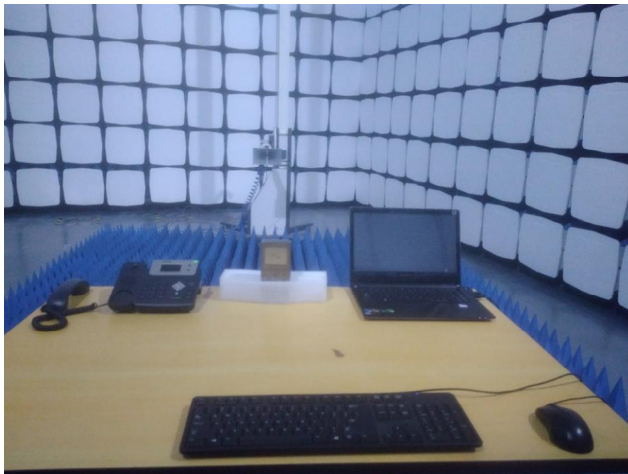
Radiated Emission test view (Above 1GHz)
