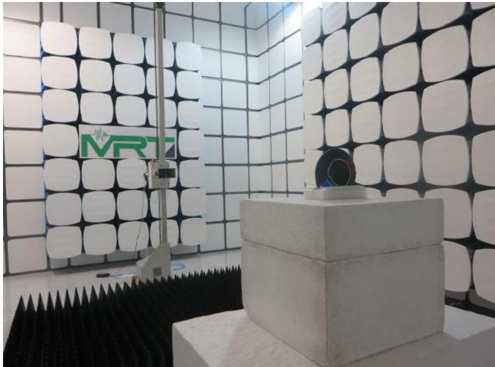
Description: Radiated Emission Test Setup for 1GHz ~ 18GHz
