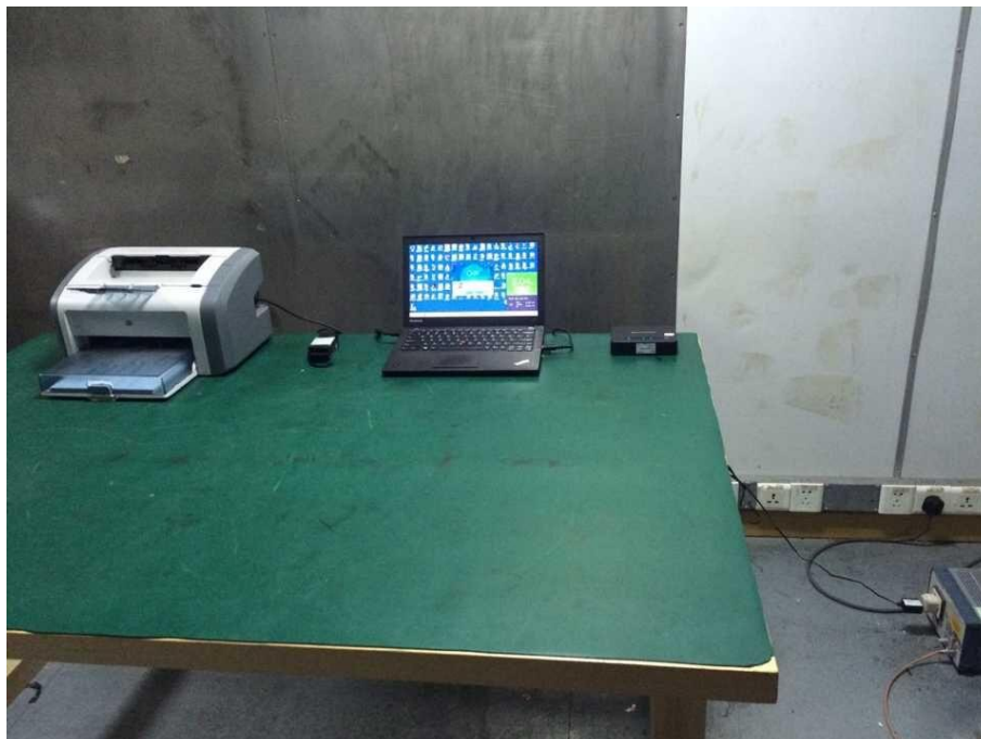
FP Conducted Emission test view
