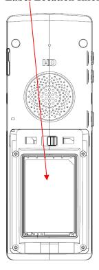
The label shown shall be permanently affixed at a conspicuous location on the device and be readily visible to the user at the time purchase (Labeling requirements per 2.925)
