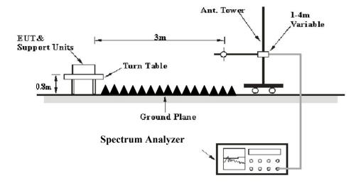
The radiated emission tests were performed in the 3 meters test site.
