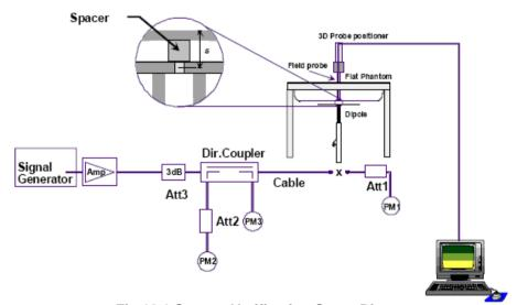
Fig.10.1 System Verification Setup Diagram
