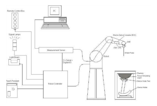
Fig. 8.1 SPEAG DASY System Configurations
