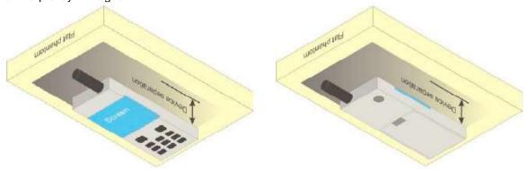
Fig.11.6 Illustration for Hotspot Position
