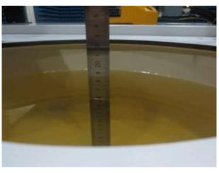
Fig. 9.2 Photo of Liquid Height for Body SAR of Twin Phantom (1900MHz) (depth>15cm)
