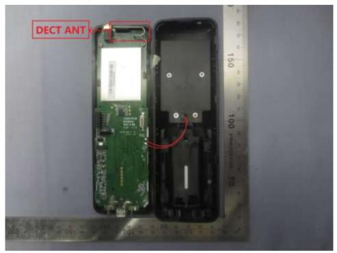
Fig.14.1 EUT Antenna Locations
