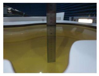
Fig. 9.1 Photo of Liquid Height for Head SAR (1900MHz) (depth>15cm)
