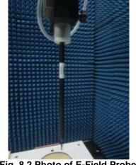
Fig. 8.2 Photo of E-Field Probe
