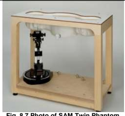
Fig. 8.7 Photo of SAM Twin Phantom
