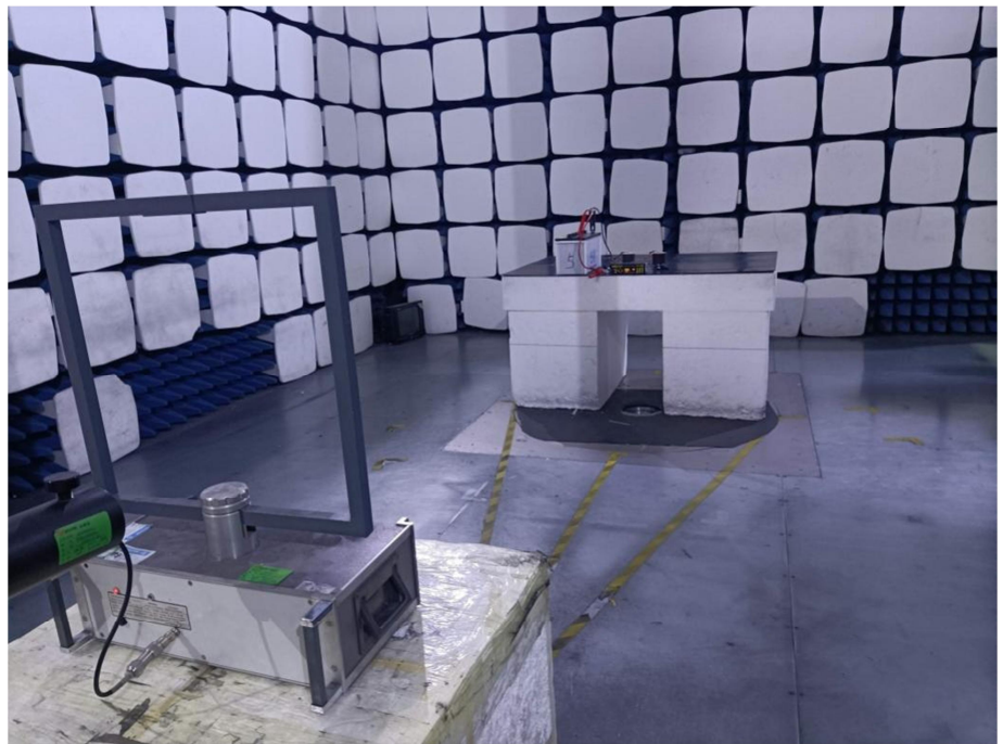
Radiation Emission Test Setup (Below 30MHz)
