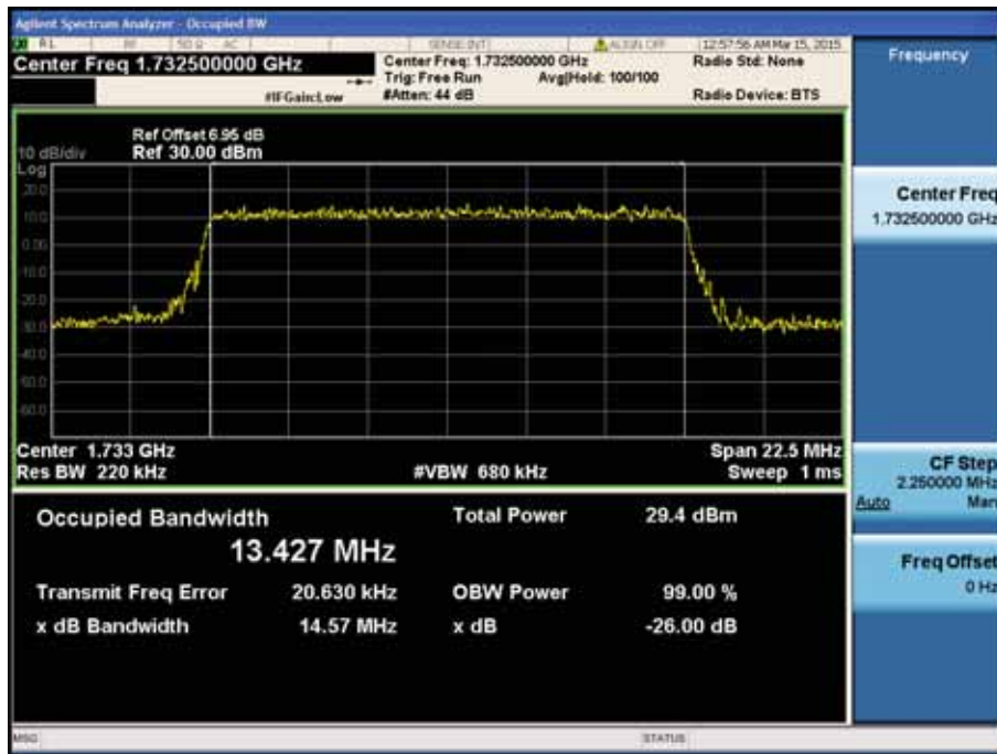
LTE Band 4 / 15MHz / QPSK - RB Size 75
