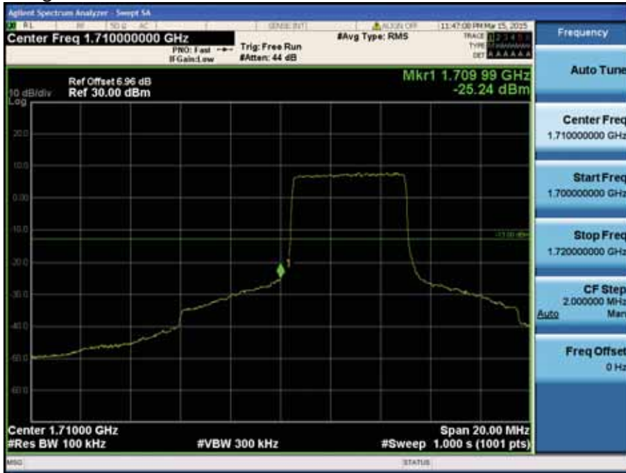
LTE Band 4 / 10MHz / QPSK - RB Size/Offset (25/0)
