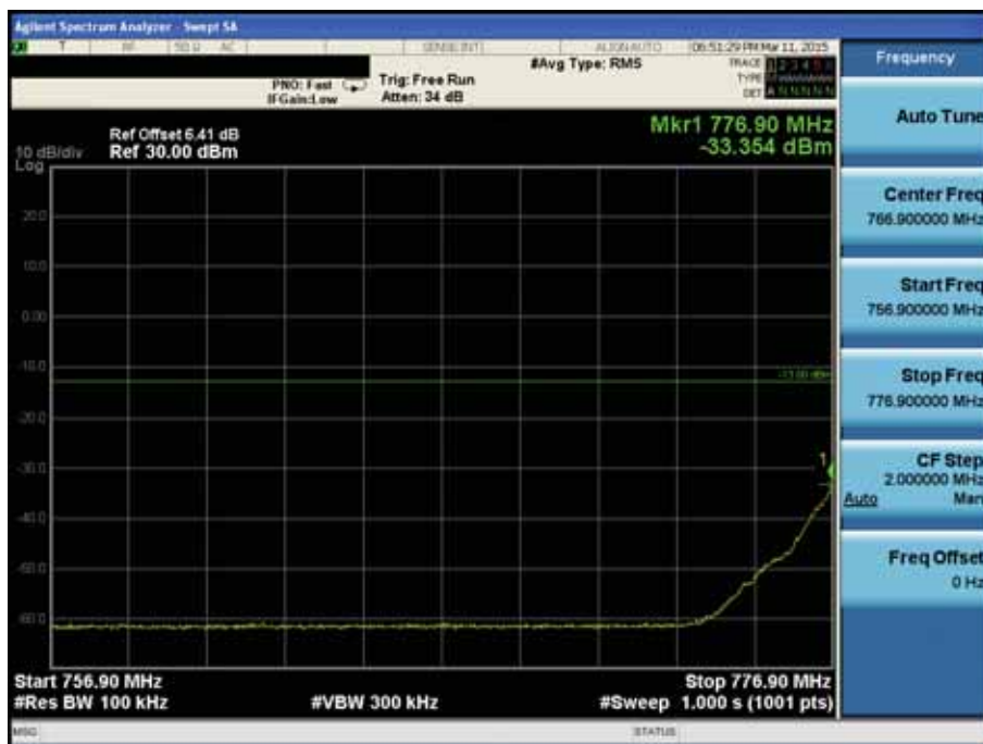
LTE Band 13 / 10MHz / QPSK - RB Size/Offset (25/0)
