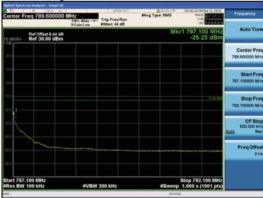
LTE Band 13 / 5MHz / 16QAM - RB Size/Offset (1/24)
