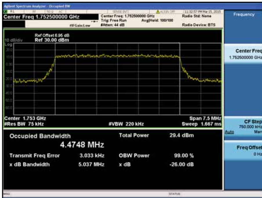
LTE Band 4 / 5MHz / QPSK - RB Size 25
