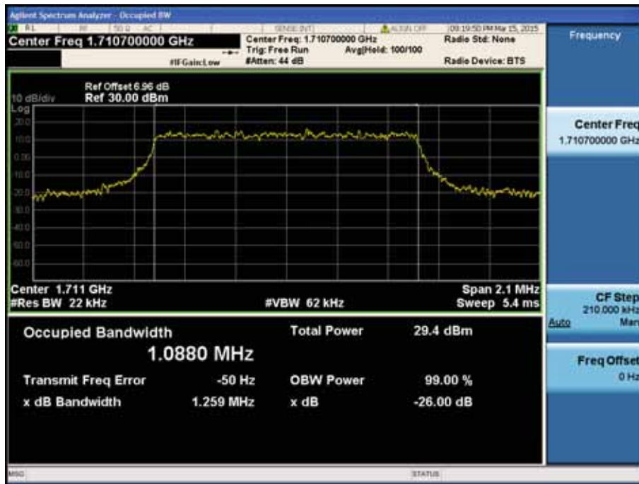
LTE Band 4 / 1.4MHz / QPSK - RB Size 6
