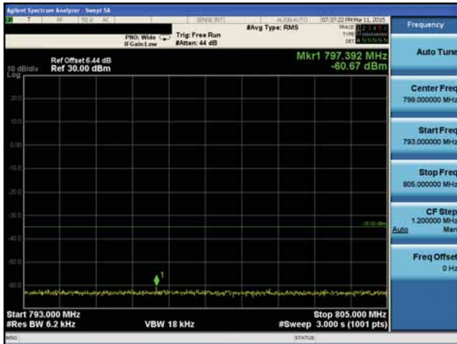
LTE Band 13 / 10MHz / QPSK - RB Size/Offset (50/0)
