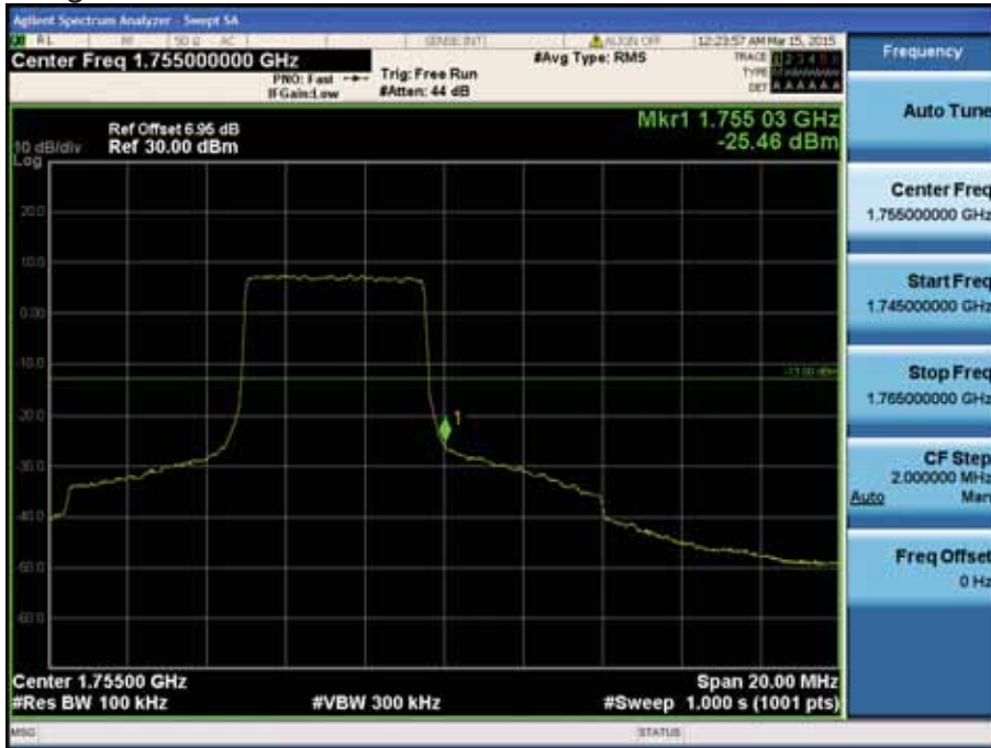
LTE Band 4 / 10MHz / QPSK - RB Size/Offset (25/25)
