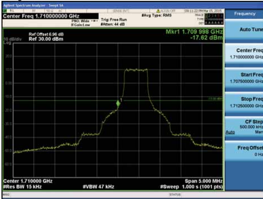
LTE Band 4 / 1.4MHz / QPSK - RB Size/Offset (3/0)
