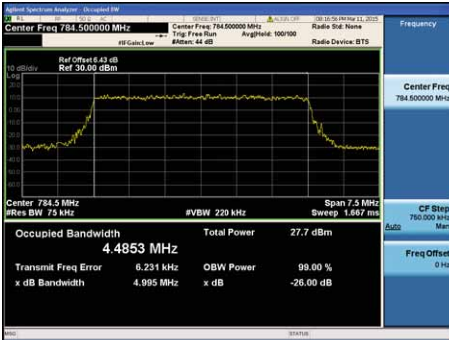
LTE Band 13 / 5MHz / 16QAM - RB Size 25
