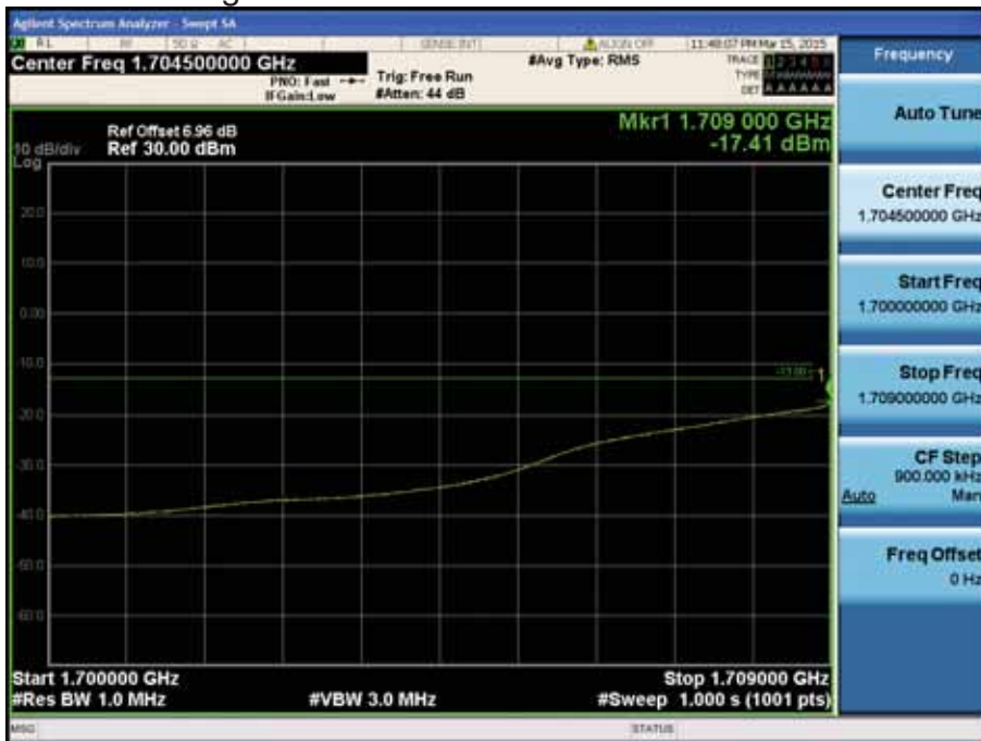
LTE Band 4 / 10MHz / QPSK - RB Size/Offset (25/0)
