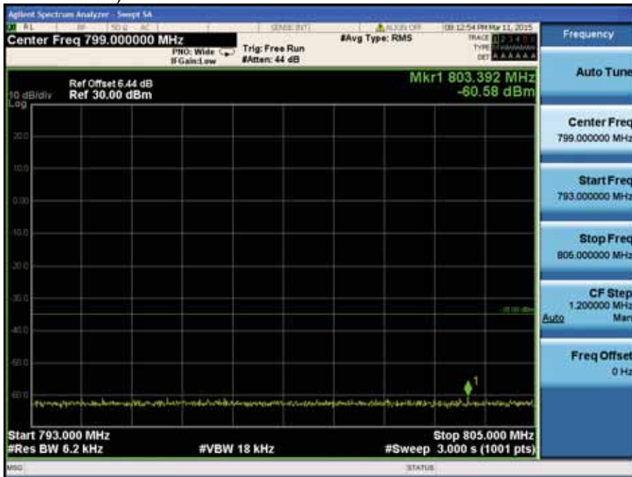
LTE Band 13 / 5MHz / 16QAM - RB Size/Offset (12/6)
