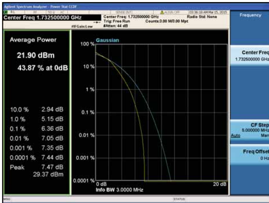
LTE Band 4 / 3MHz / 16QAM - RB Size 15
