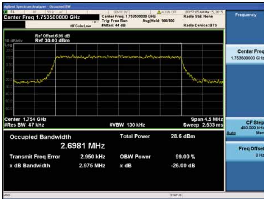
LTE Band 4 / 3MHz / 16QAM - RB Size 15
