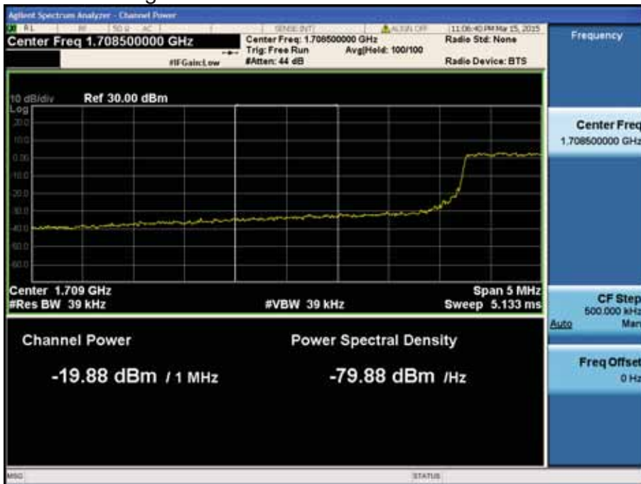
LTE Band 4 / 5MHz / QPSK - RB Size/Offset (25/0)
