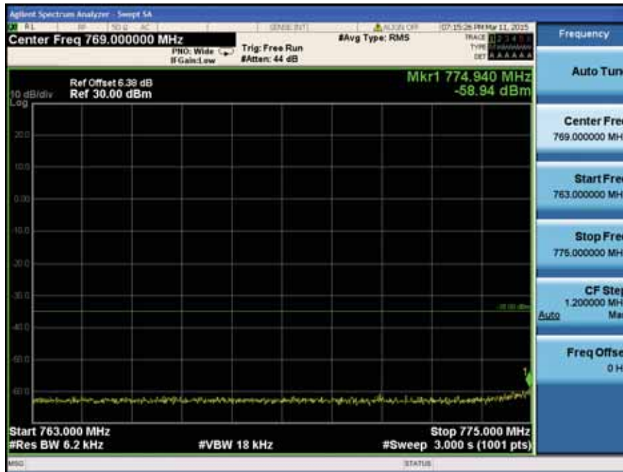
LTE Band 13 / 10MHz / QPSK - RB Size/Offset (25/0)
