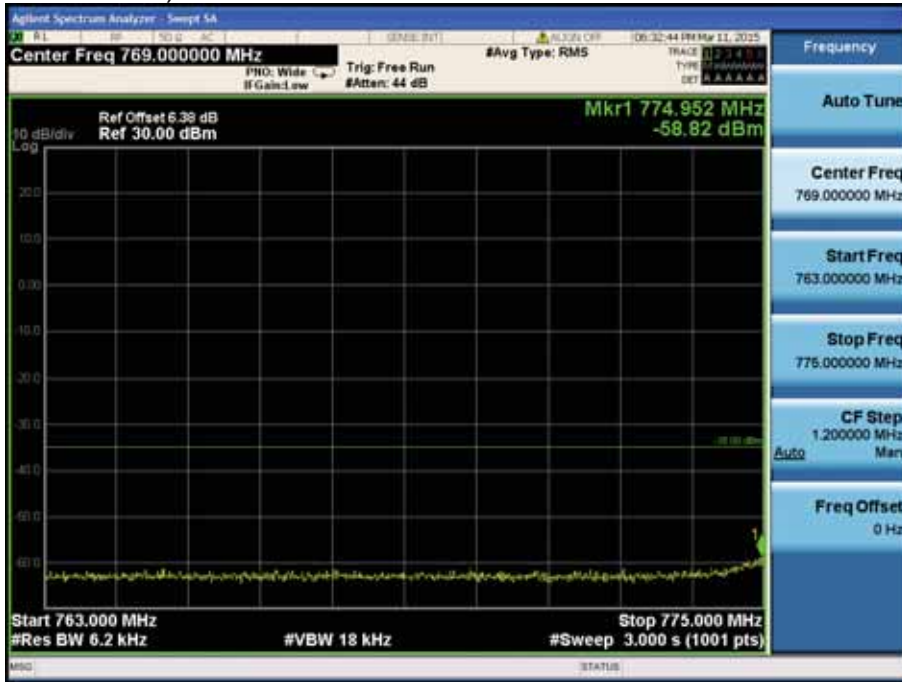
LTE Band 13 / 5MHz / QPSK - RB Size/Offset (25/0)
