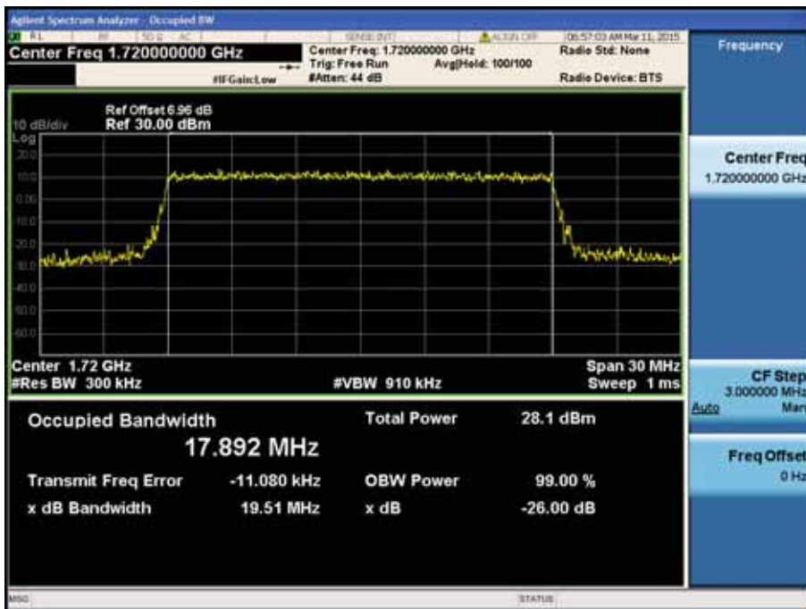
LTE Band 4 / 20MHz / 16QAM - RB Size 100
