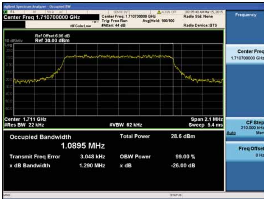
LTE Band 4 / 1.4MHz / 16QAM - RB Size 6
