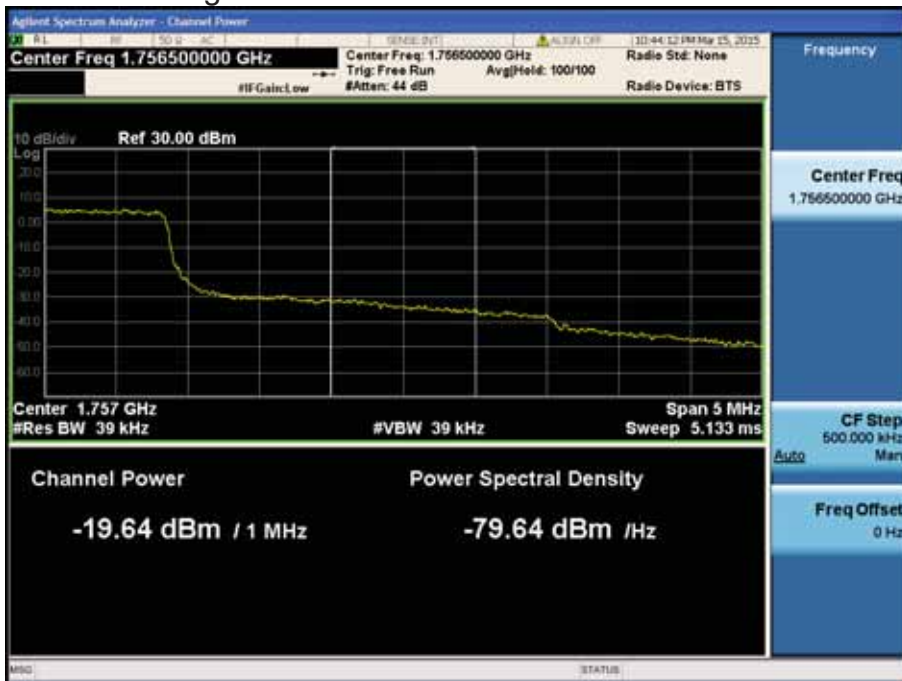
LTE Band 4 / 3MHz / QPSK - RB Size/Offset (15/0)
