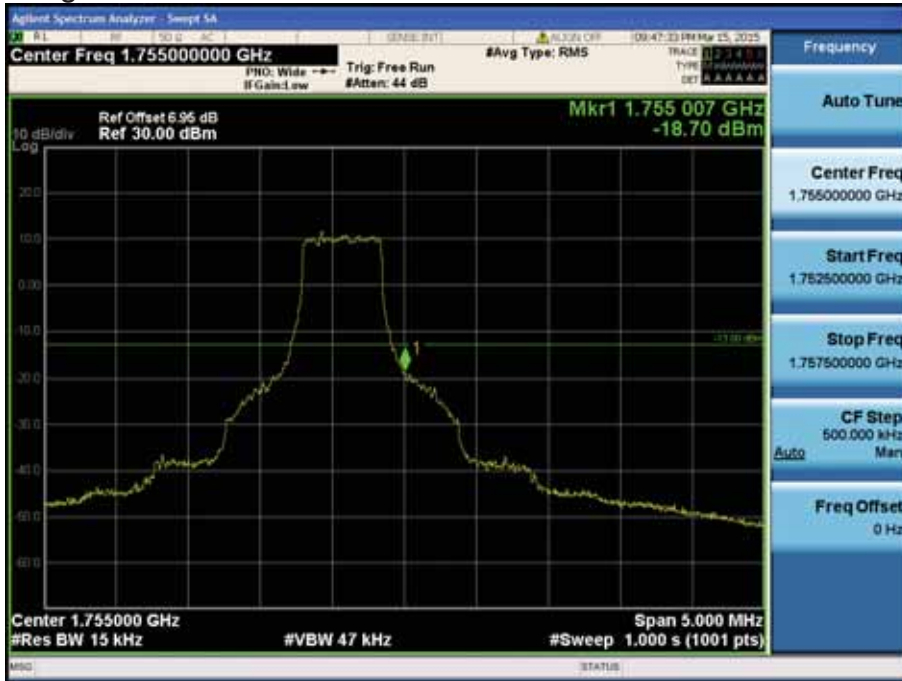
LTE Band 4 / 1.4MHz / QPSK - RB Size/Offset (3/3)
