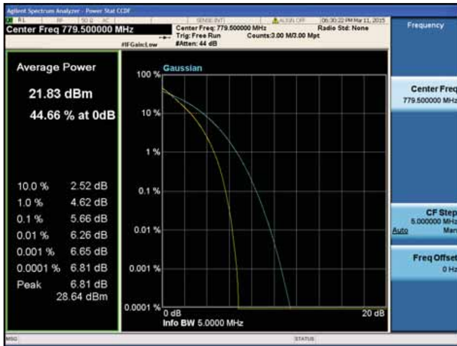
LTE Band 13 / 5MHz / QPSK - RB Size 25
