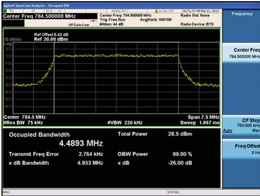
LTE Band 13 / 5MHz / QPSK - RB Size 25
