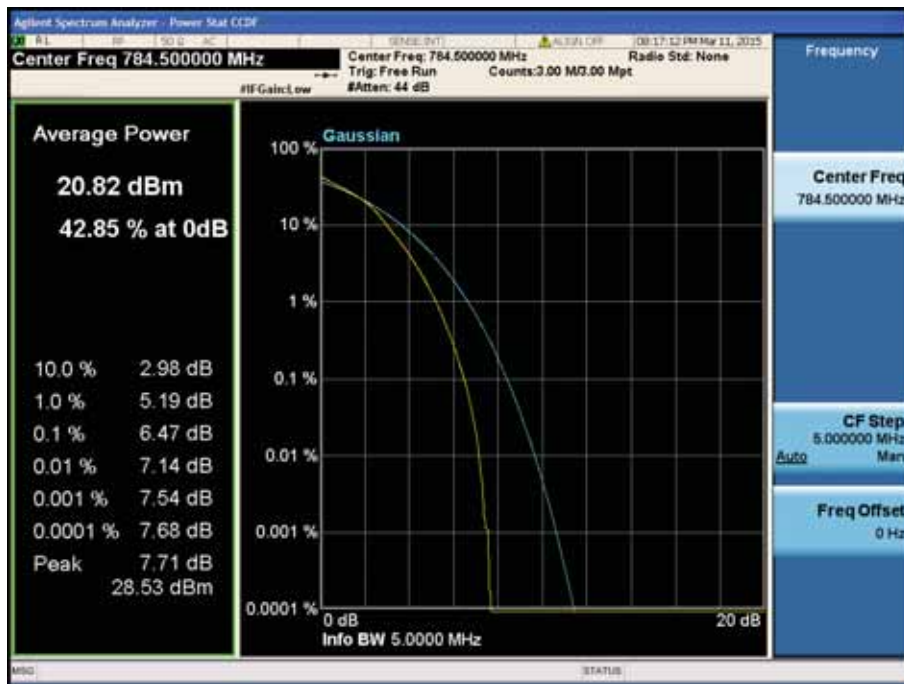
LTE Band 13 / 5MHz / 16QAM - RB Size 25
