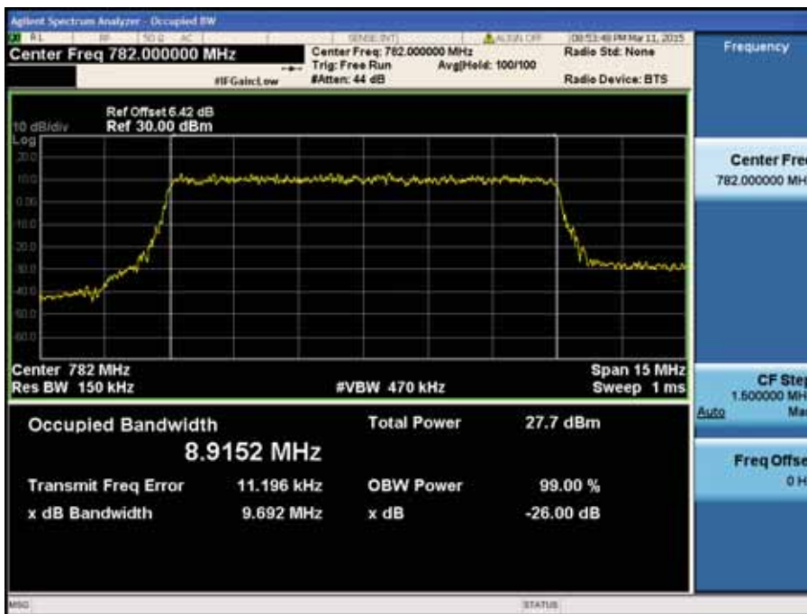
LTE Band 13 / 10MHz / 16QAM - RB Size 50
