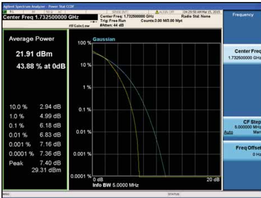
LTE Band 4 / 5MHz / 16QAM - RB Size 25
