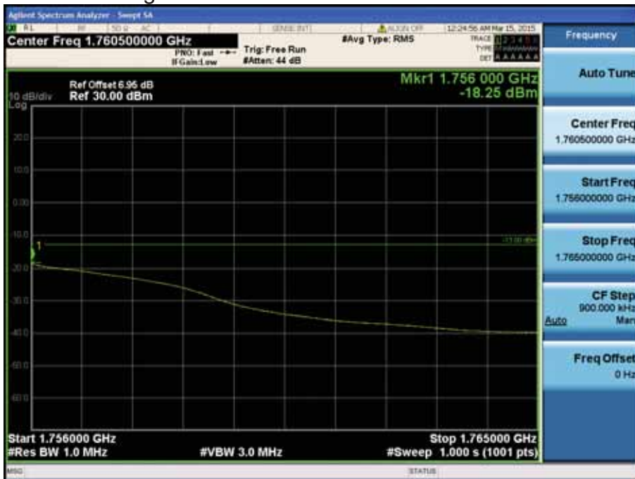
LTE Band 4 / 10MHz / QPSK - RB Size/Offset (25/25)
