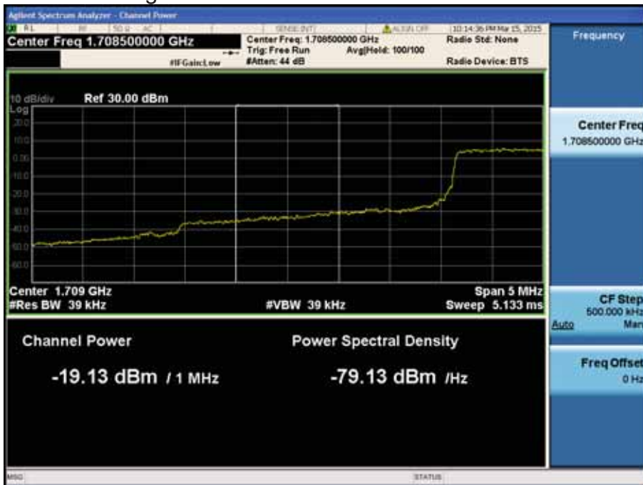
LTE Band 4 / 3MHz / QPSK - RB Size/Offset (15/0)
