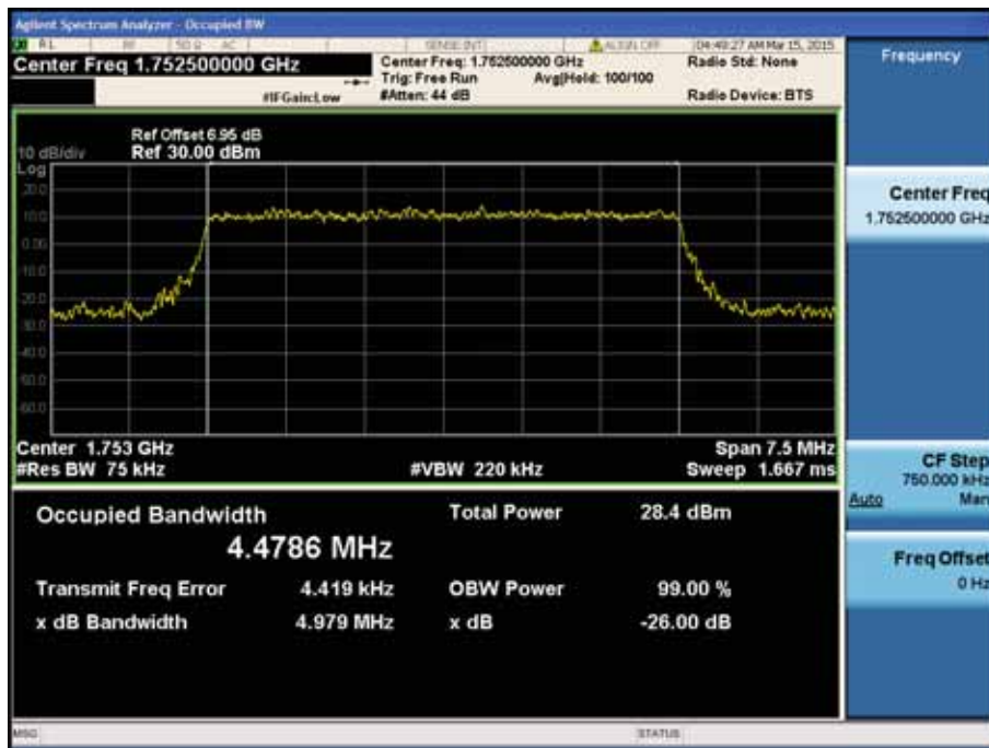
LTE Band 4 / 5MHz / 16QAM - RB Size 25
