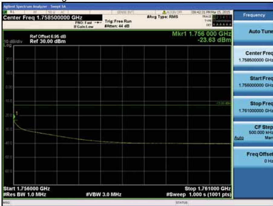
LTE Band 4 / 1.4MHz / QPSK - RB Size/Offset (3/0)
