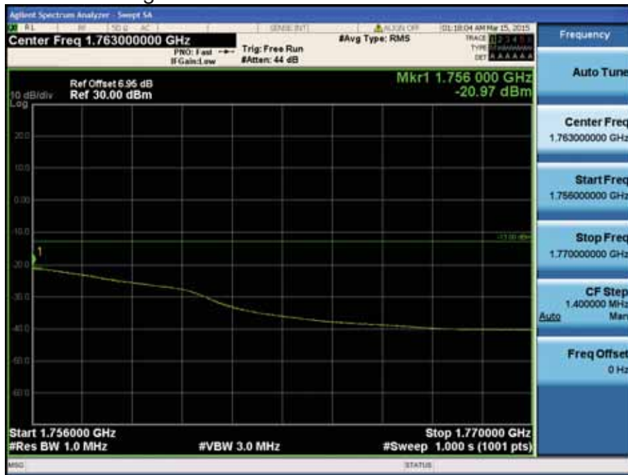
LTE Band 4 / 15MHz / QPSK - RB Size/Offset (36/39)
