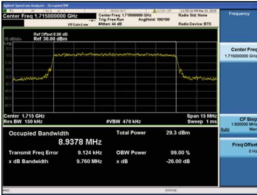
LTE Band 4 / 10MHz / QPSK - RB Size 50
