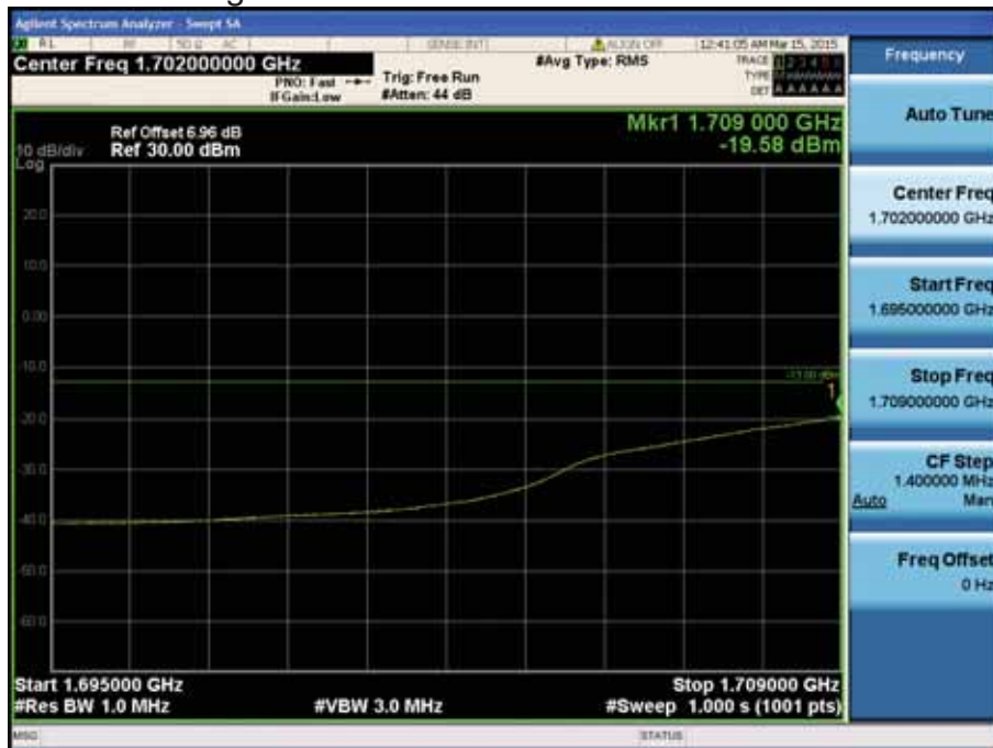
LTE Band 4 / 15MHz / QPSK - RB Size/Offset (36/0)
