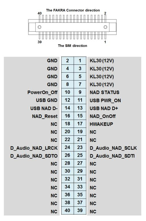
Figure 1. Connector pin arrangement
