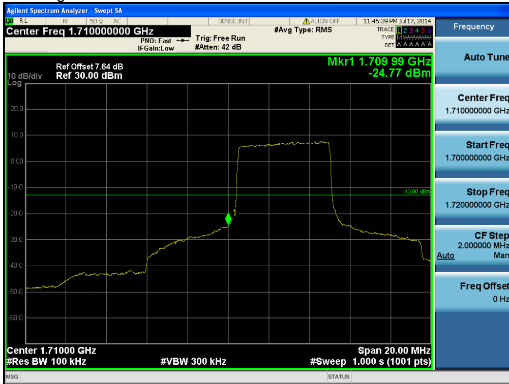
LTE Band 4 / 10MHz / QPSK - RB Offset/Size (0/25)
