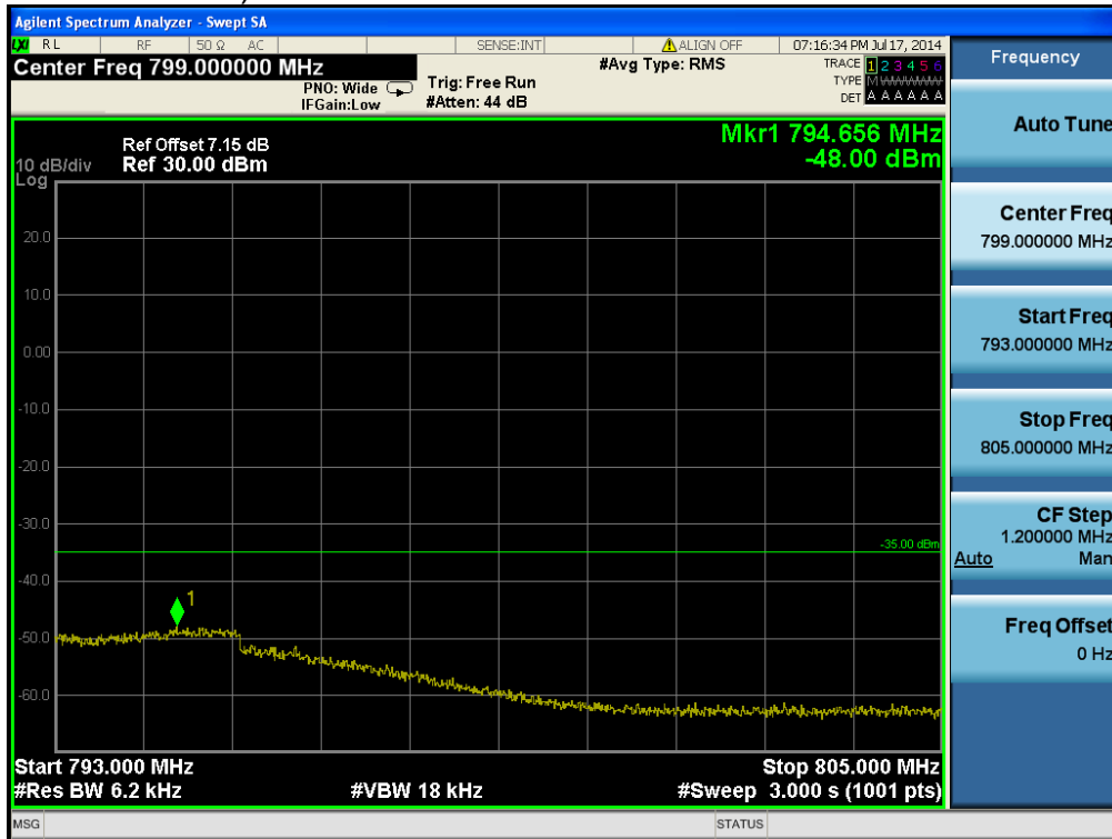
LTE Band 13 / 10MHz / QPSK - Offset/Size (0/50)
