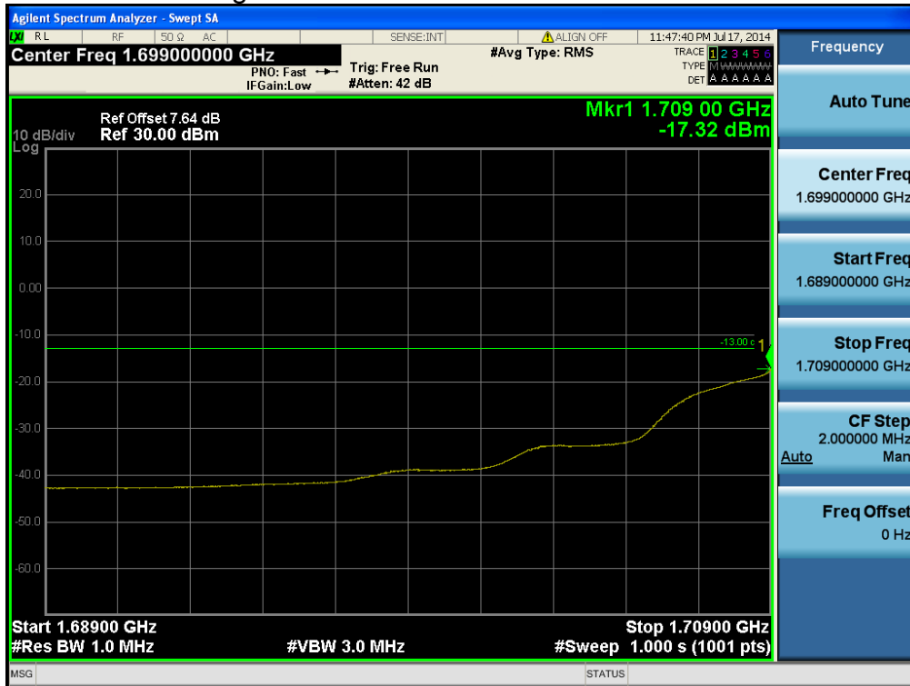
LTE Band 4 / 10MHz / QPSK - RB Offset/Size (0/25)
