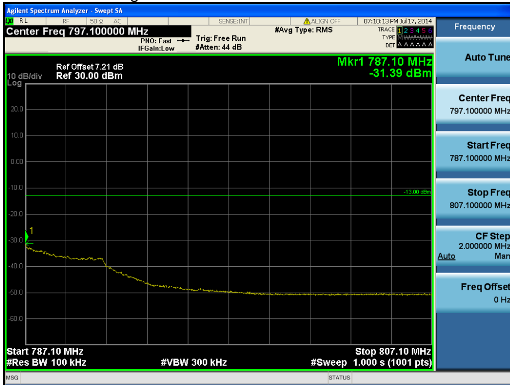
LTE Band 13 / 10MHz / QPSK - RB Offset/Size (12/25)
