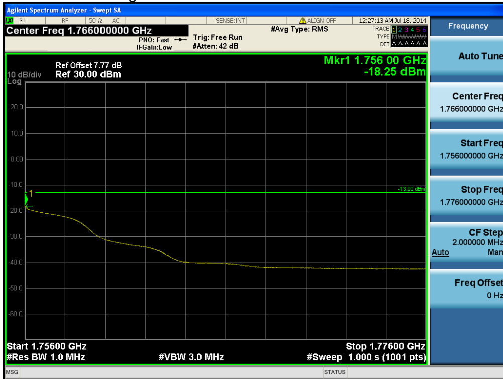
LTE Band 4 / 10MHz / QPSK - RB Offset/Size (25/25)
