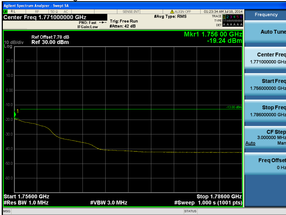
LTE Band 4 / 15MHz / QPSK - RB Offset/Size (39/36)
