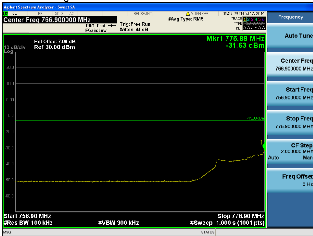
LTE Band 13 / 10MHz / QPSK - RB Offset/Size (0/25)
