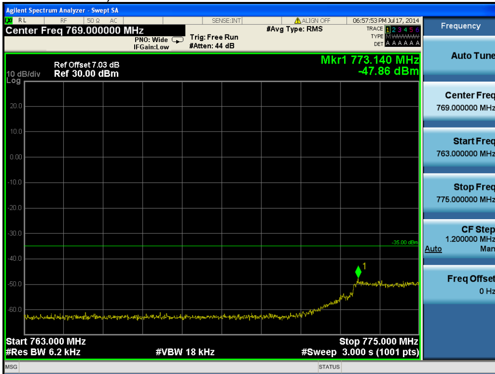
LTE Band 13 / 10MHz / QPSK - RB Offset/Size (0/25)
