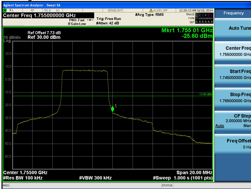
LTE Band 4 / 10MHz / QPSK - RB Offset/Size (25/25)
