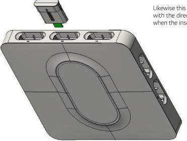
Likewise this picture, when you inserting modules, be careful with the directions. Modules will not be able to be putted in when the inserting direction is opposite.
