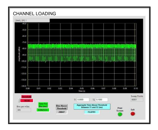
The level of traffic loading on the channel by the EUT is 73.07%
