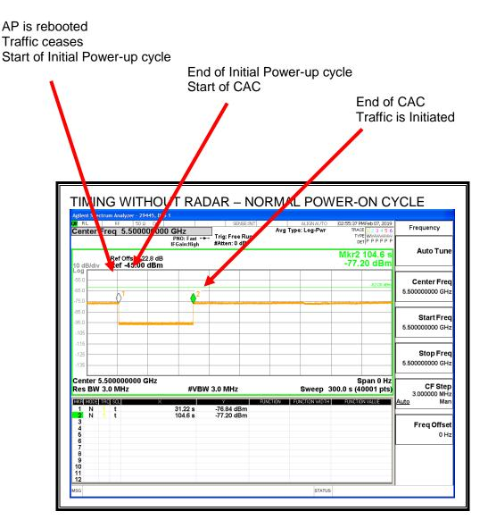
Transmissions begin on channel after completion of the initial power-up cycle and the CAC.
