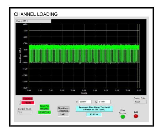
The level of traffic loading on the channel by the EUT is 75.87%
