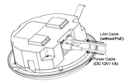
! WARRING – **Do not connect both POE cable and DC cable to ESL Gateway** (It may cause break down or fire)
