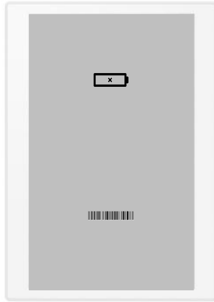
Battery discharge (The battery needs to be replaced)
