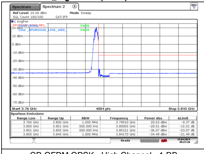
CP-OFDM QPSK - High Channel - 1 RB
