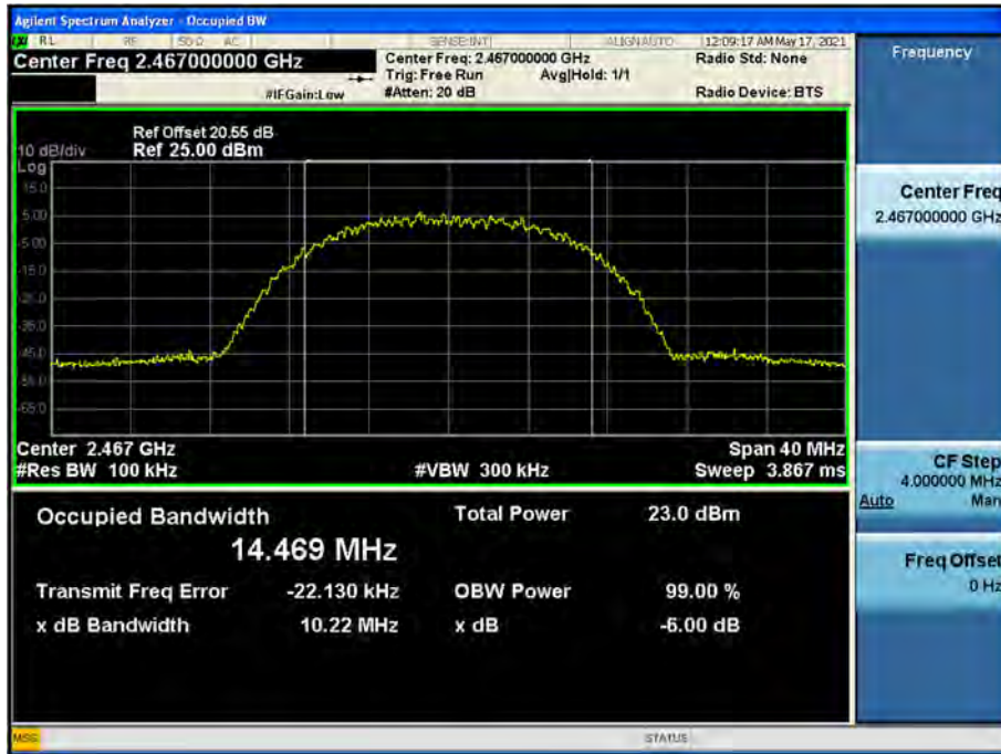
6dB Bandwidth plot (802.11b-CH 12)
