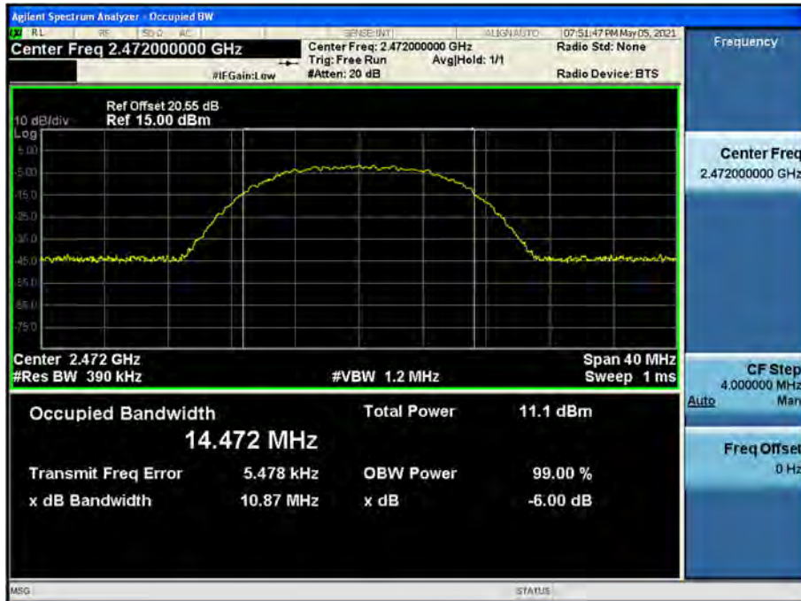
99% Bandwidth plot (802.11b-CH 13)
