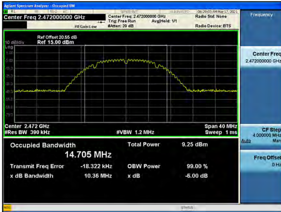
99% Bandwidth plot (802.11b-CH 13)
