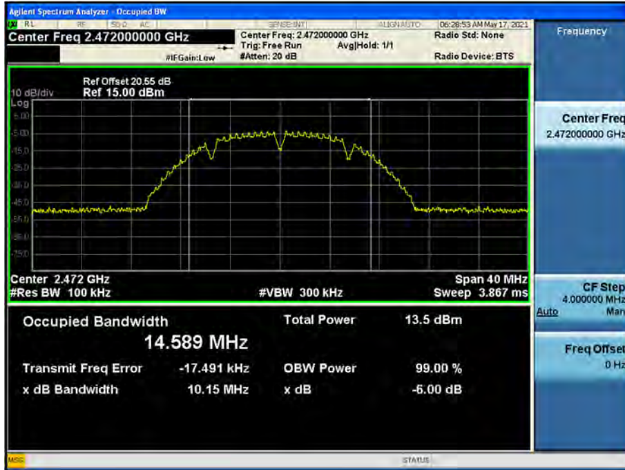
6dB Bandwidth plot (802.11b-CH 13)
