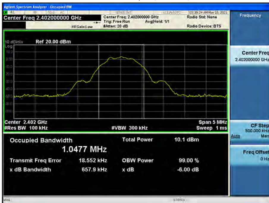
6 dB Bandwidth plot (Mid-CH 19)
