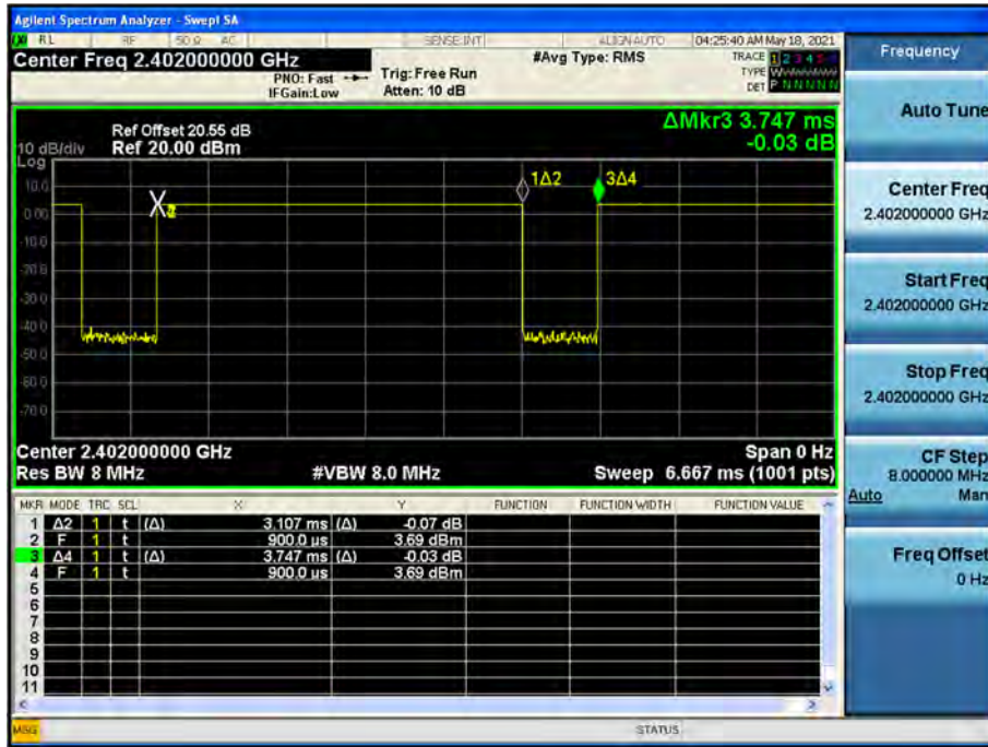
Duty Cycle (Low-CH 0)
