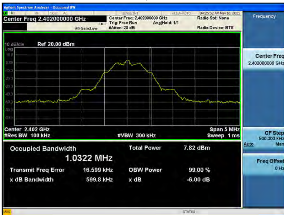
6 dB Bandwidth plot (Mid-CH 19)
