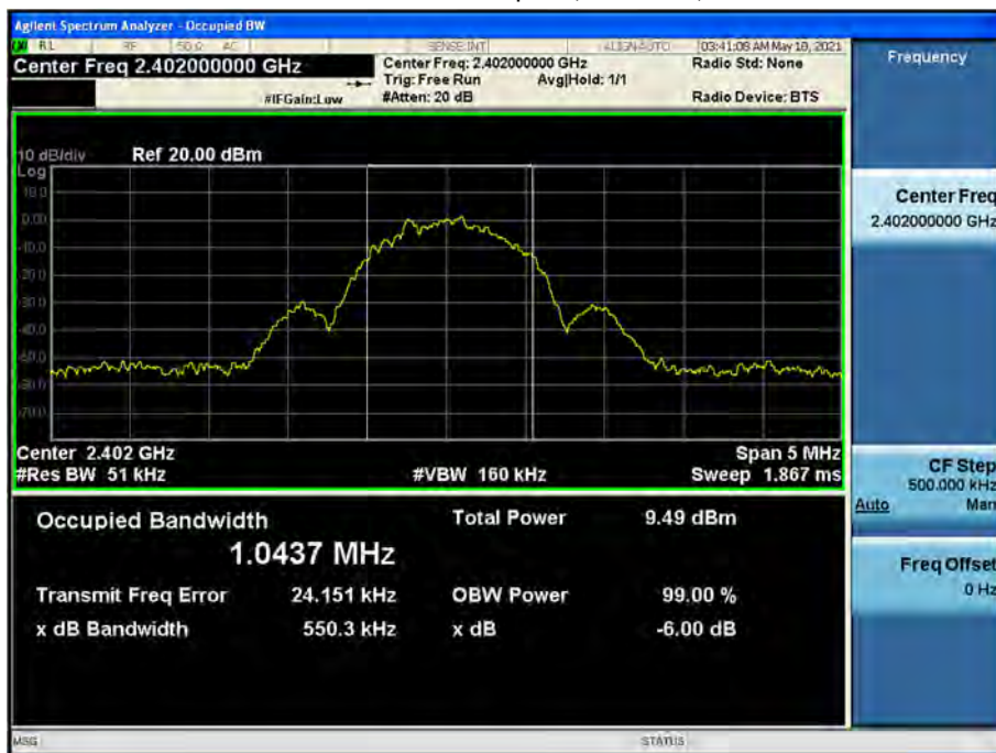
99 % Bandwidth plot (Low-CH 0)
