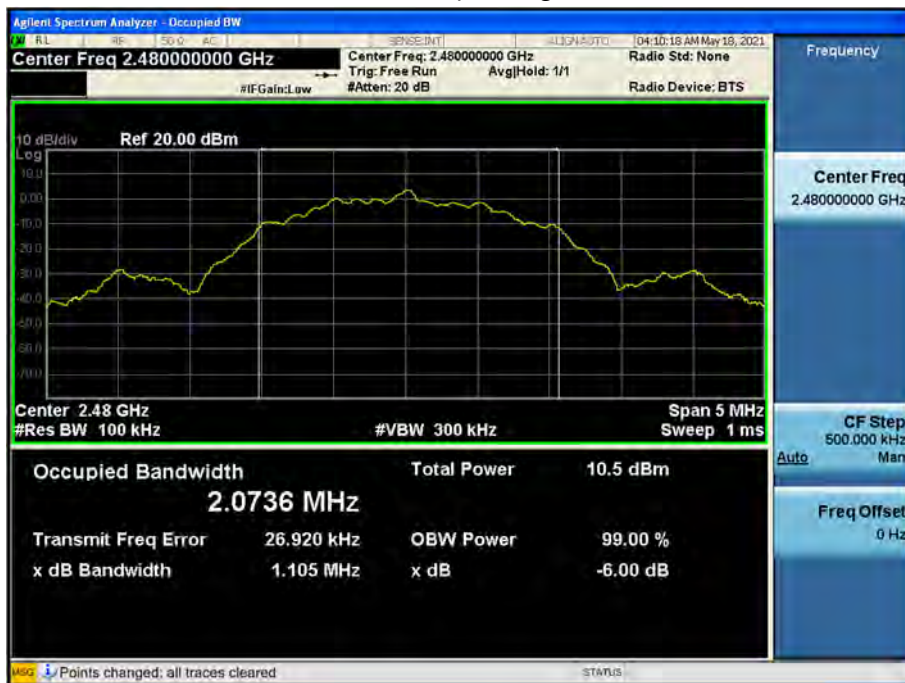
6 dB Bandwidth plot (High-CH 39)
