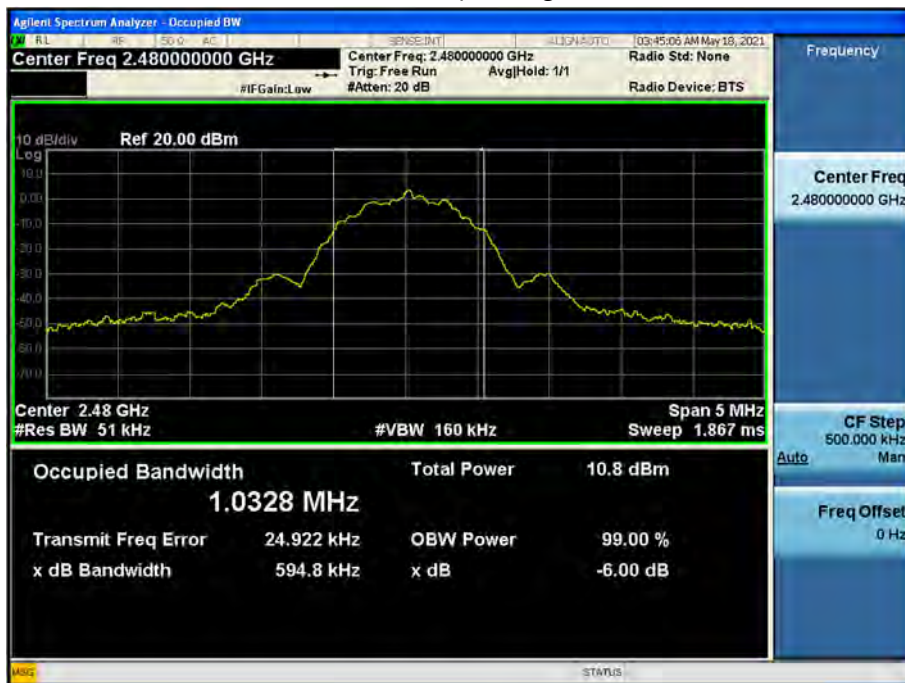
99 % Bandwidth plot (High-CH 39)
