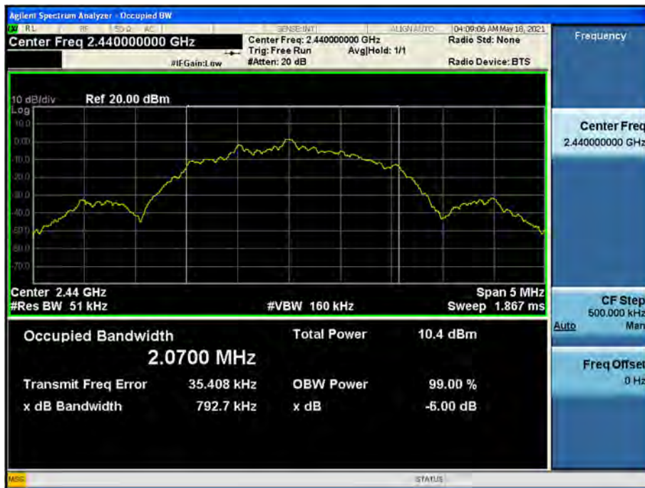
99 % Bandwidth plot (Mid-CH 19)
