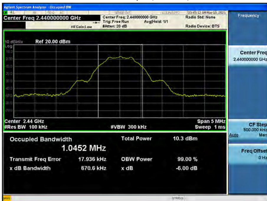
6 dB Bandwidth plot (Mid-CH 19)
