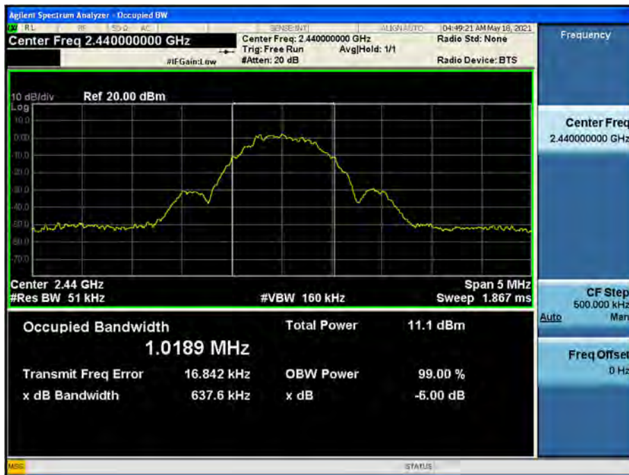
99 % Bandwidth plot (Mid-CH 19)
