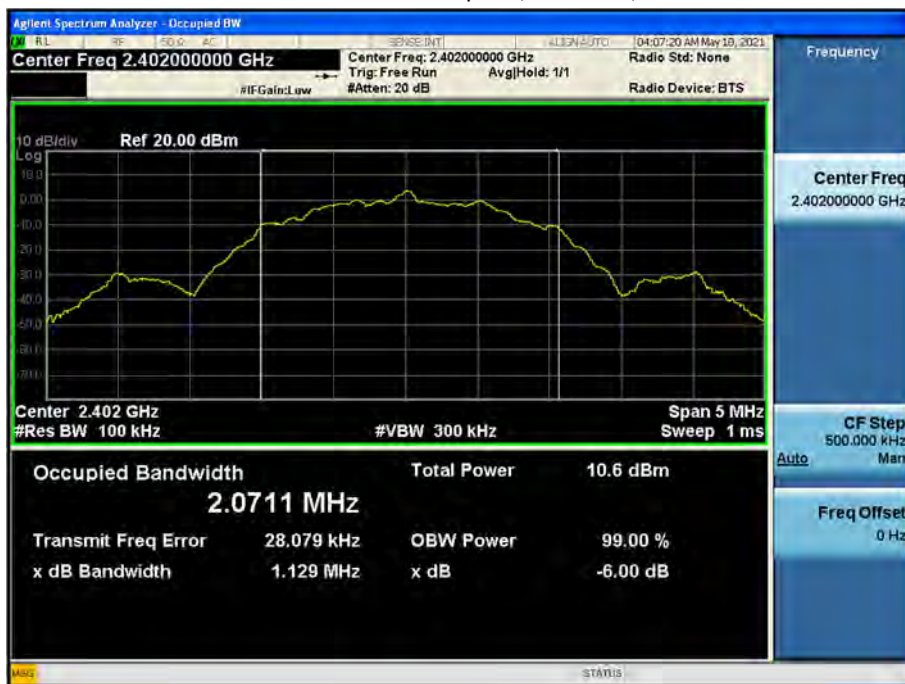
6 dB Bandwidth plot (Mid-CH 19)
