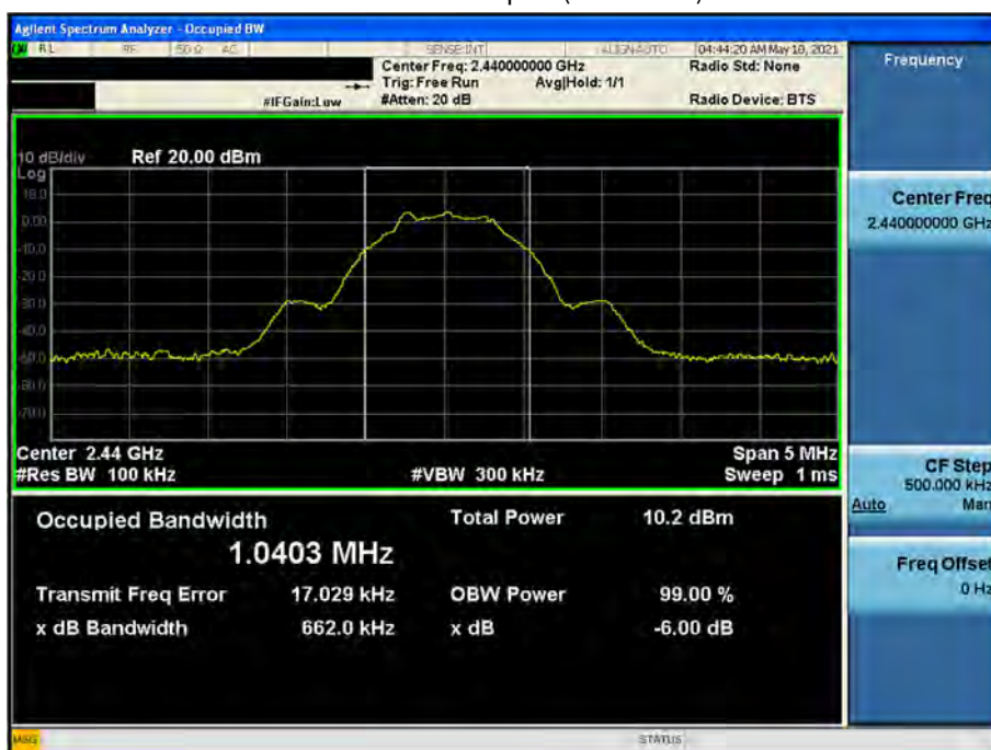
6 dB Bandwidth plot (Mid-CH 19)
