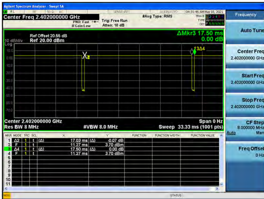
Duty Cycle (Low-CH 0)
