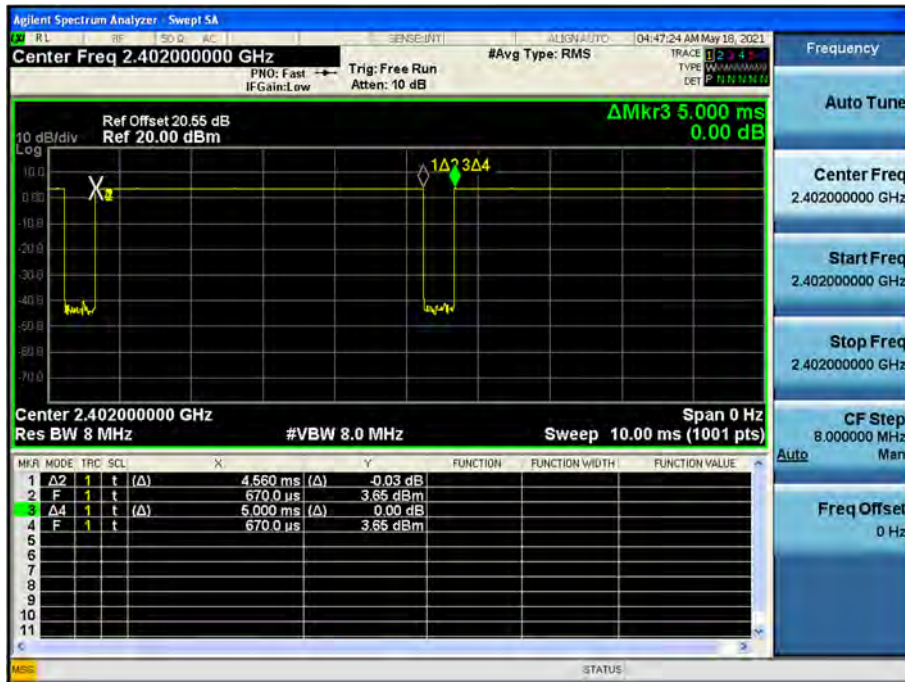
Duty Cycle (Low-CH 0)
