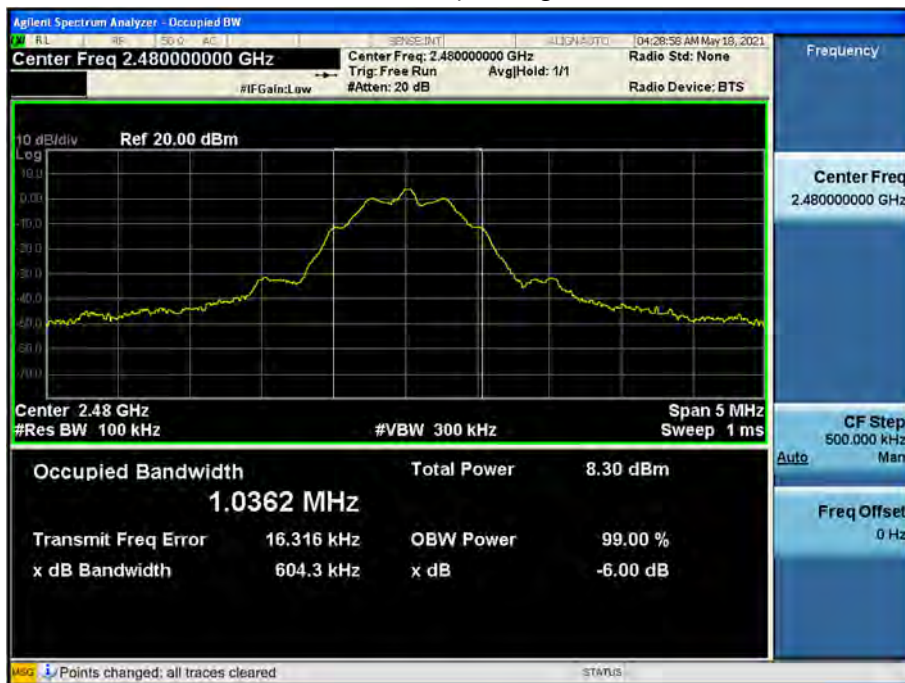
6 dB Bandwidth plot (High-CH 39)
