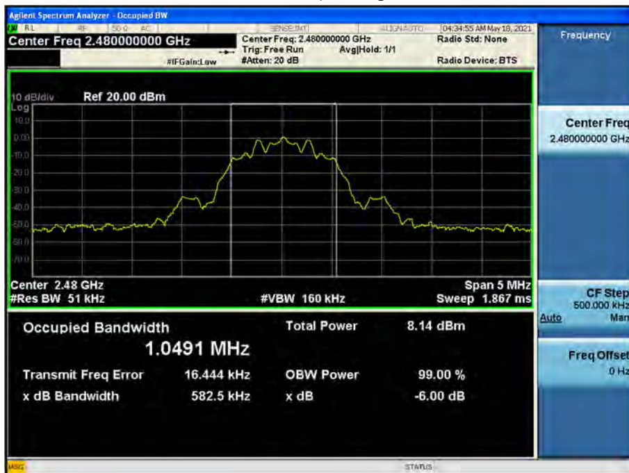
99 % Bandwidth plot (High-CH 39)
