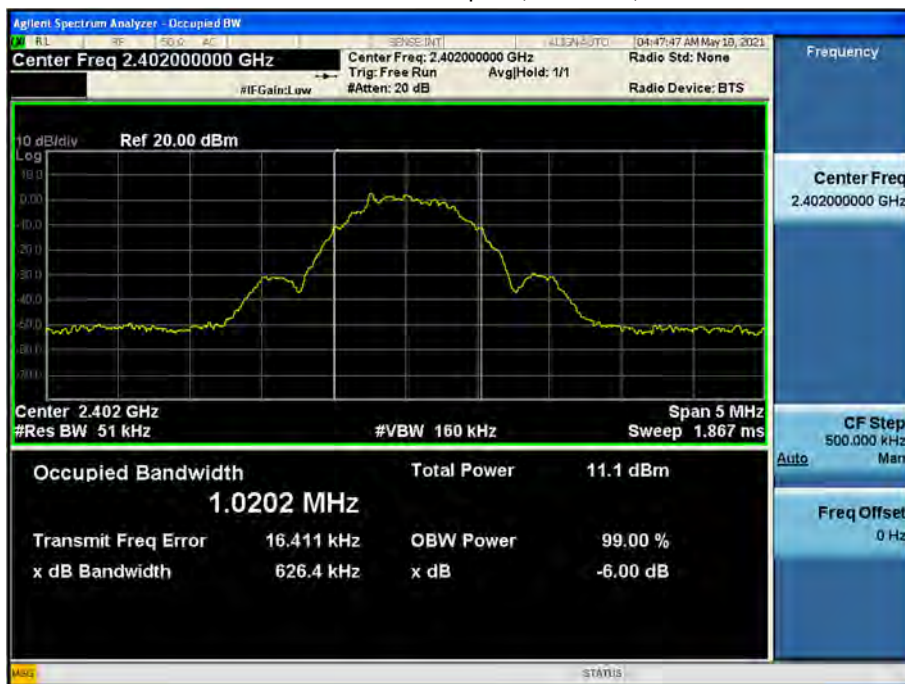
99 % Bandwidth plot (Low-CH 0)
