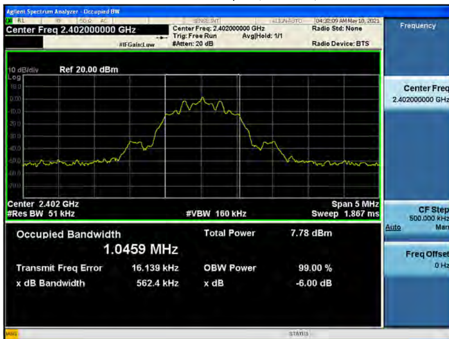
99 % Bandwidth plot (Low-CH 0)
