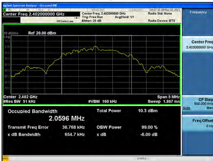
99 % Bandwidth plot (Low-CH 0)
