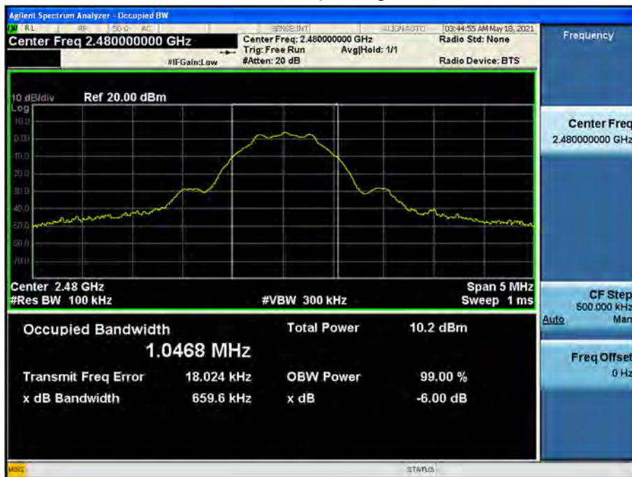
6 dB Bandwidth plot (High-CH 39)
