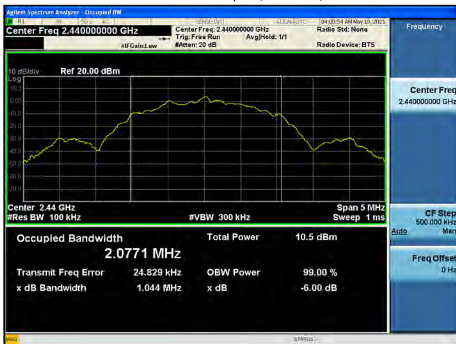
6 dB Bandwidth plot (Mid-CH 19)
