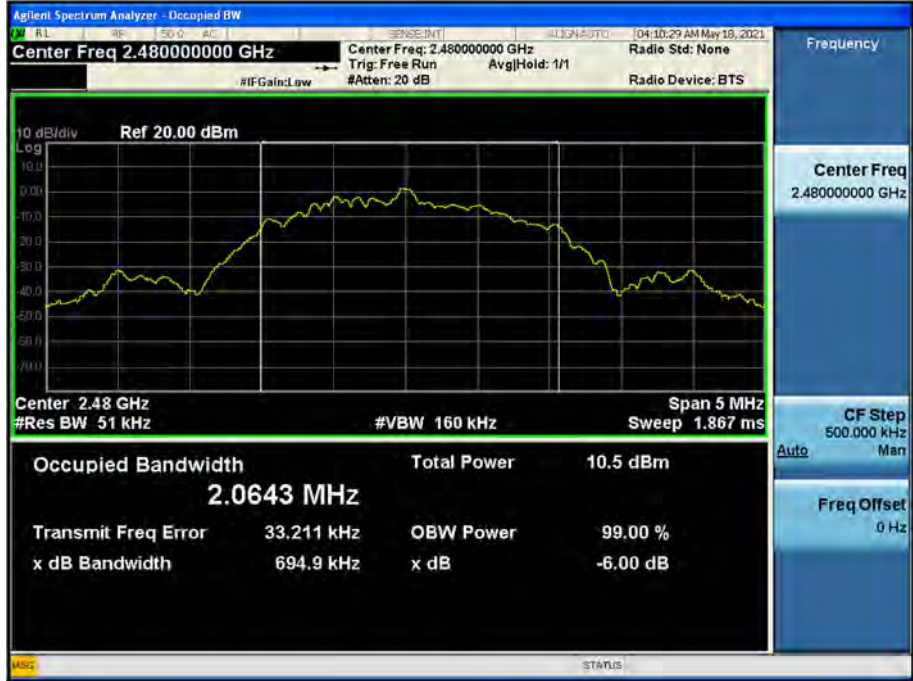
99 % Bandwidth plot (High-CH 39)
