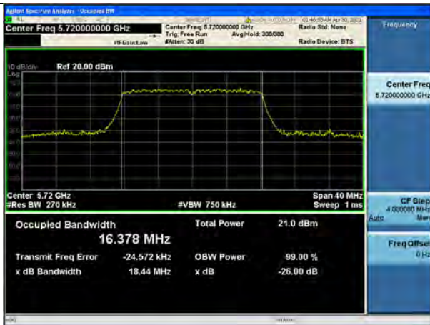
802.11a UNII 2C BAND 26dB Bandwidth (CH 144)
