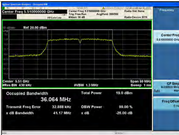
802.11ac_VHT40 UNII 2C BAND 26dB Bandwidth(CH 102)
