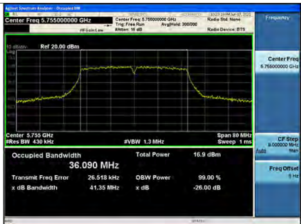
802.11n_HT40 UNII 3 BAND 26dB Bandwidth (CH 151)
