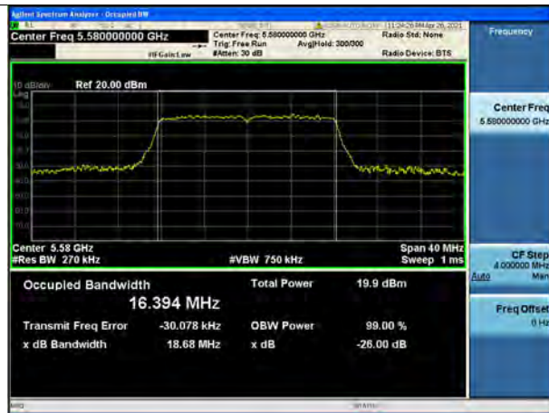
802.11a UNII 2C BAND 26dB Bandwidth (CH116)
