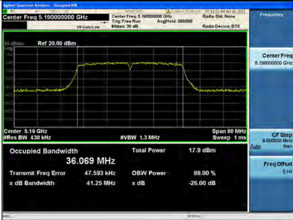
802.11ac_VHT40 UNII 2C BAND 26dB Bandwidth(CH 102)
