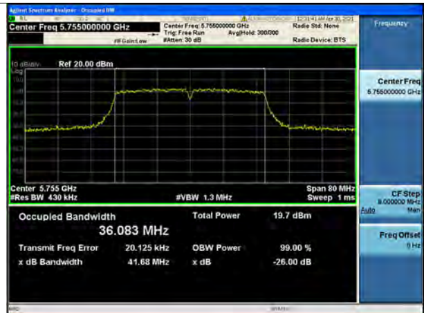
802.11ac_VHT40 UNII 3 BAND 26dB Bandwidth (CH 151)
