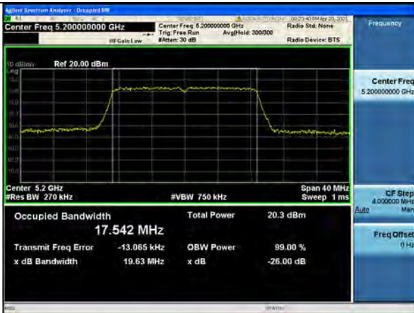
802.11n_HT20 UNII 2C BAND 26dB Bandwidth(CH 144)
