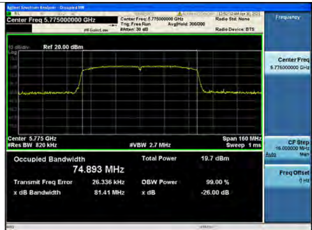
802.11ac_VHT80 UNII 3 BAND 26dB Bandwidth (CH 155)
