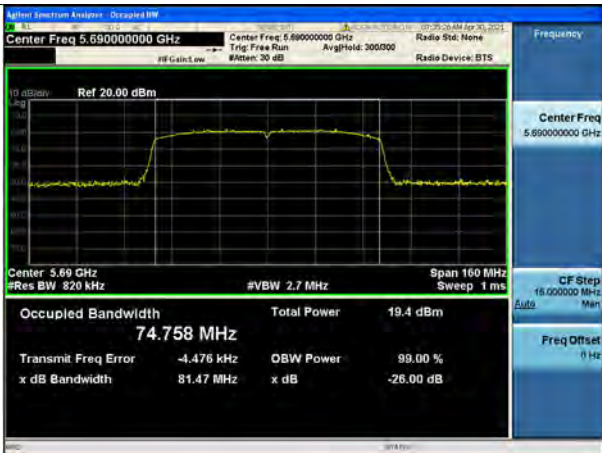
802.11ac_VHT80 UNII 2C BAND 26dB Bandwidth(CH 138)
