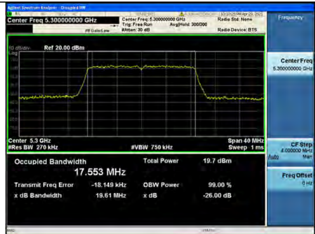
802.11n_HT20 UNII 3 BAND 26dB Bandwidth(CH 157)
