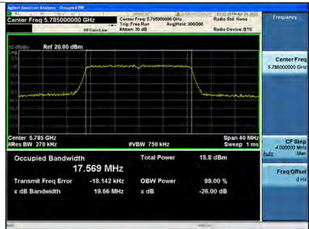
802.11n_HT20 UNII 3 BAND 26dB Bandwidth(CH 157)
