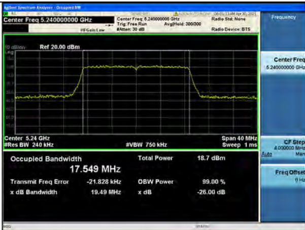
802.11n_HT20 UNII 2C BAND 26dB Bandwidth(CH 116)
