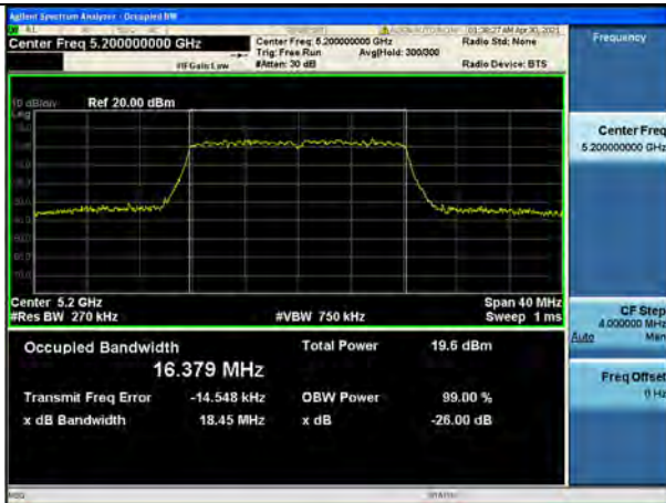
802.11a UNII 2C BAND 26dB Bandwidth (CH 144)
