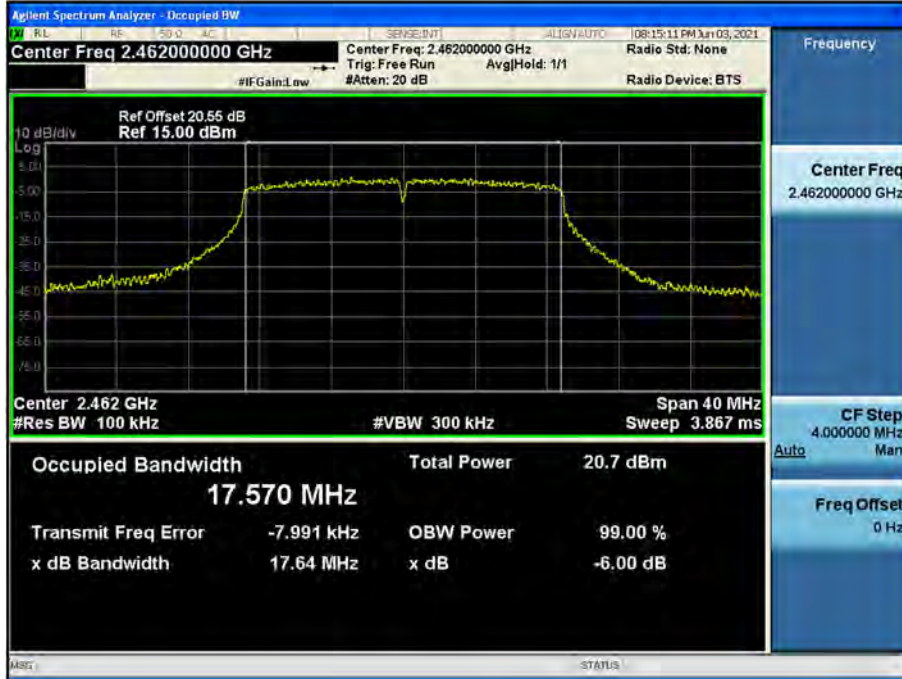
6dB Bandwidth plot (802.11n_HT20-CH 11)
