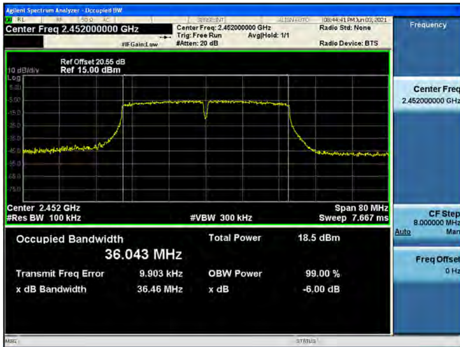
6dB Bandwidth plot (802.11n_HT40-CH 9)
