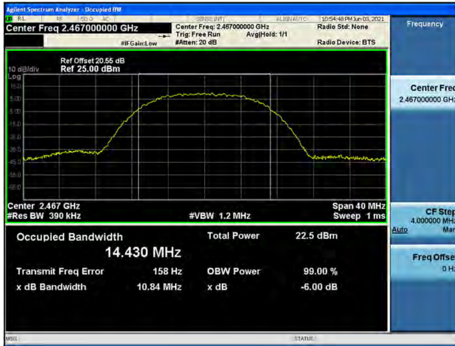
99% Bandwidth plot (802.11b-CH 12)
