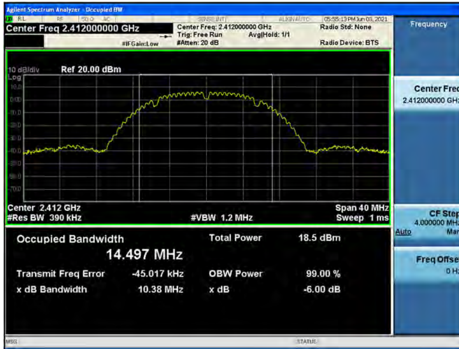
99% Bandwidth plot (802.11b-CH 1)
