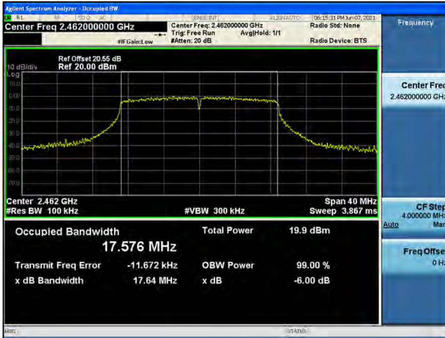
6dB Bandwidth plot (802.11n_HT20-CH 11)
