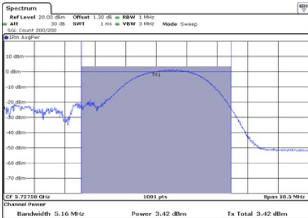
2 Stardle Maximum Conducted Output Power_UNII2C
