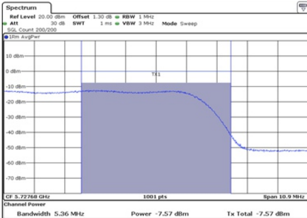
12 Staddle Maximum Conducted Output Power_UNII2C
