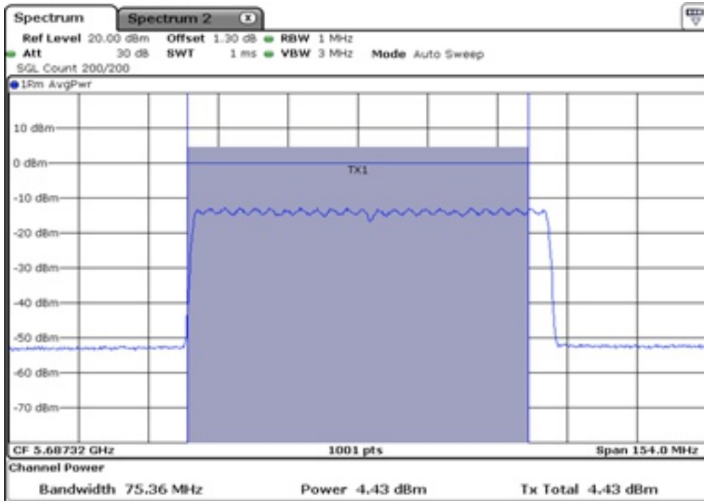
13 Staddle Maximum Conducted Output Power_UNII2C
