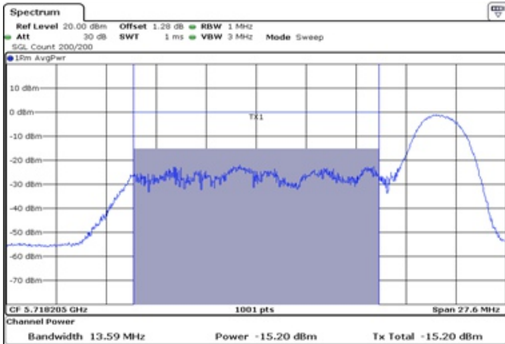
5 Starddle Maximum Conducted Output Power_UNII2C
