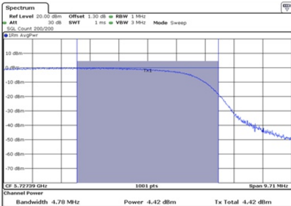
6 Staddle Maximum Conducted Output Power_UNII2C
