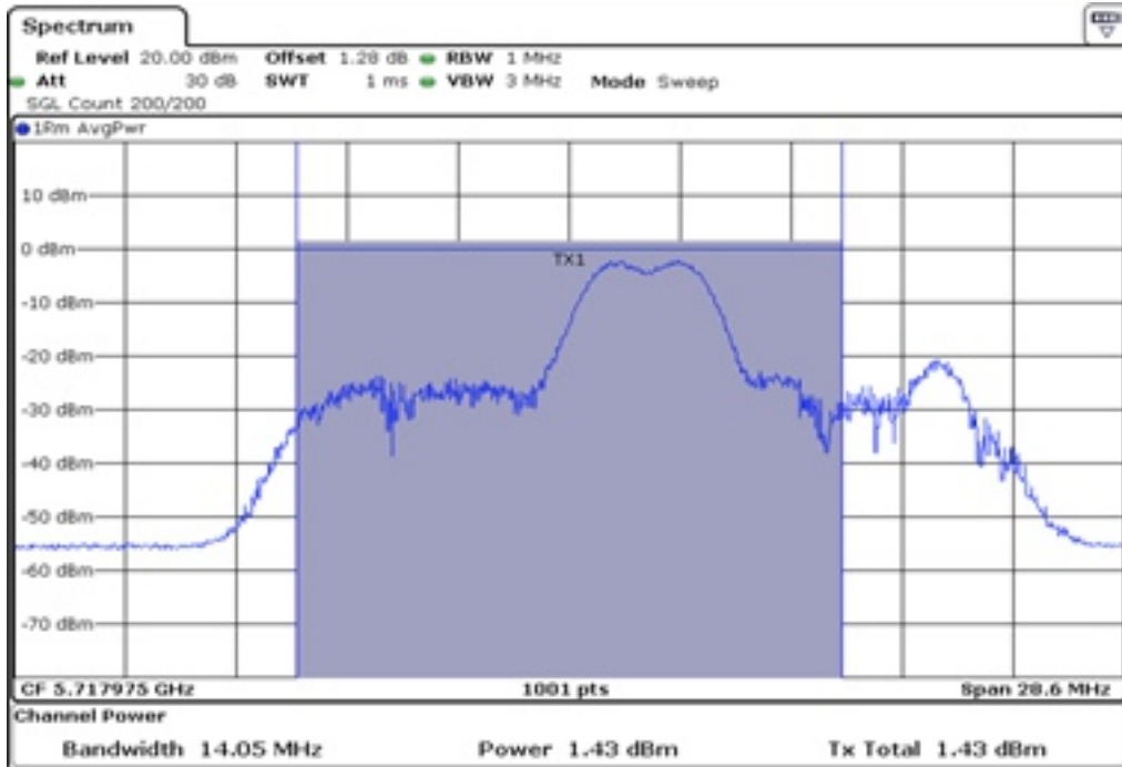
3 Stardle Maximum Conducted Output Power_UNII2C
