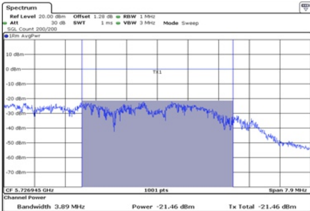
4 Stardle Maximum Conducted Output Power_UNII3
