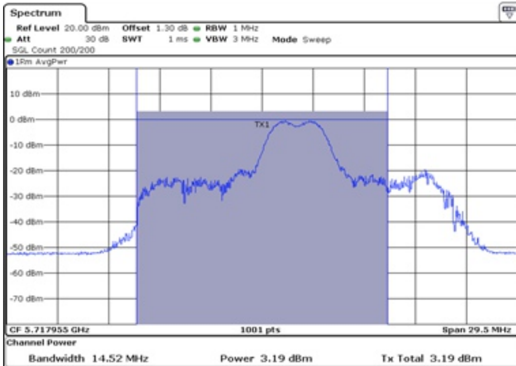
3 Stardle Maximum Conducted Output Power_UNII2C
