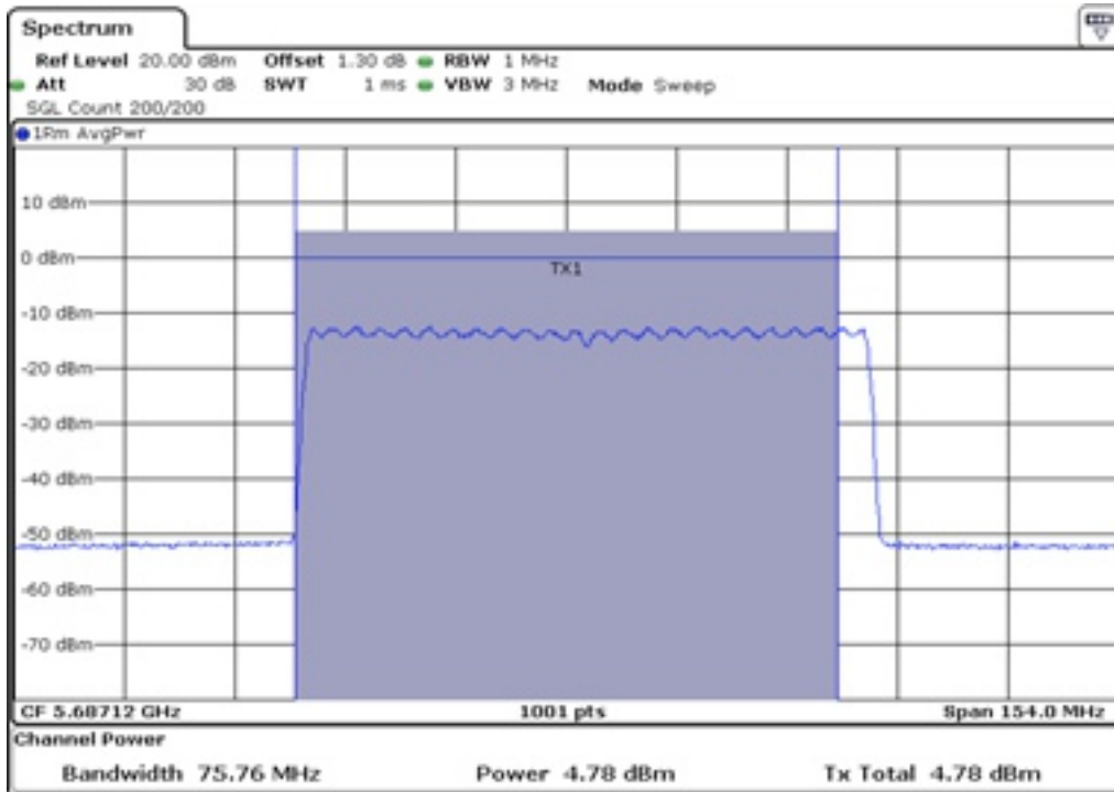
11 Staddle Maximum Conducted Output Power_UNII2C
