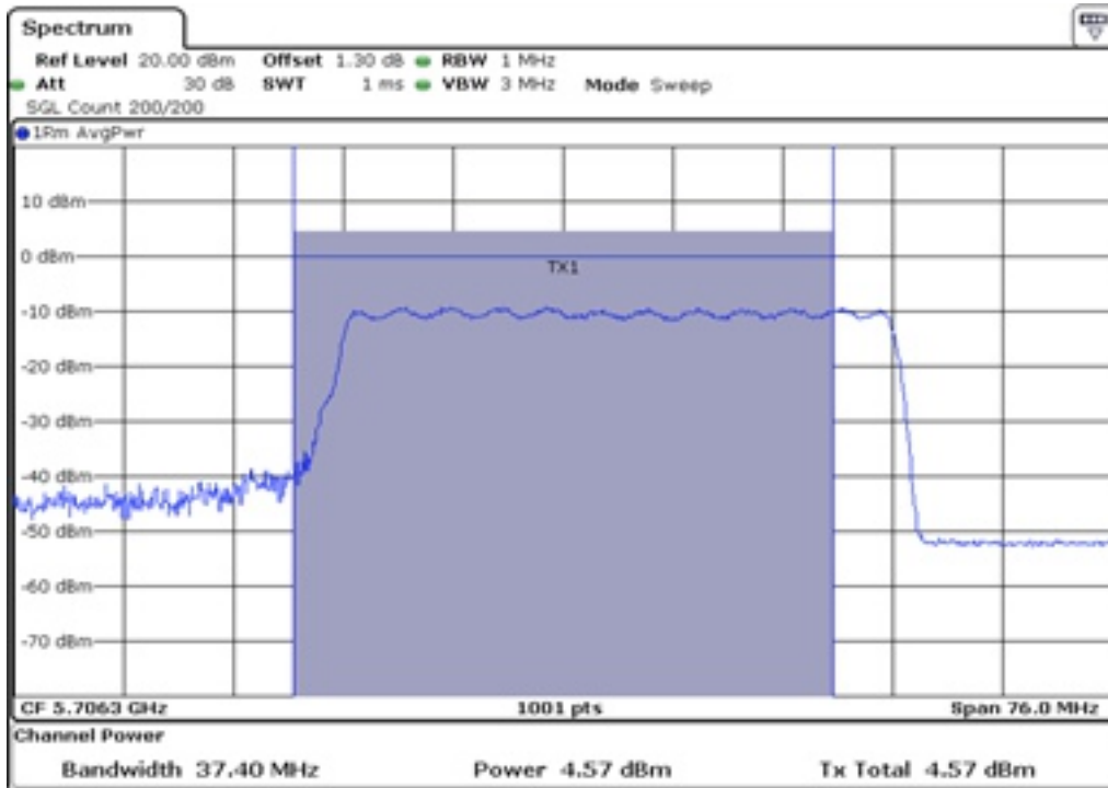
9 Stardle Maximum Conducted Output Power_UNII2C
