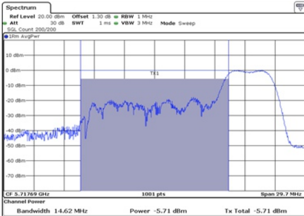
3 Starddle Maximum Conducted Output Power_UNII2C
