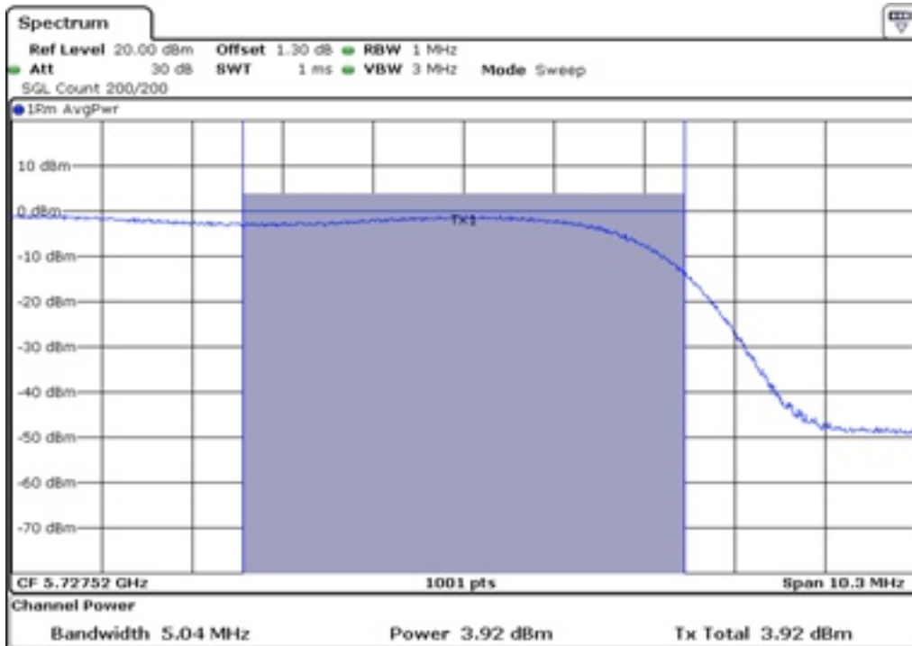
18 Staddle Maximum Conducted Output Power_UNII2C
