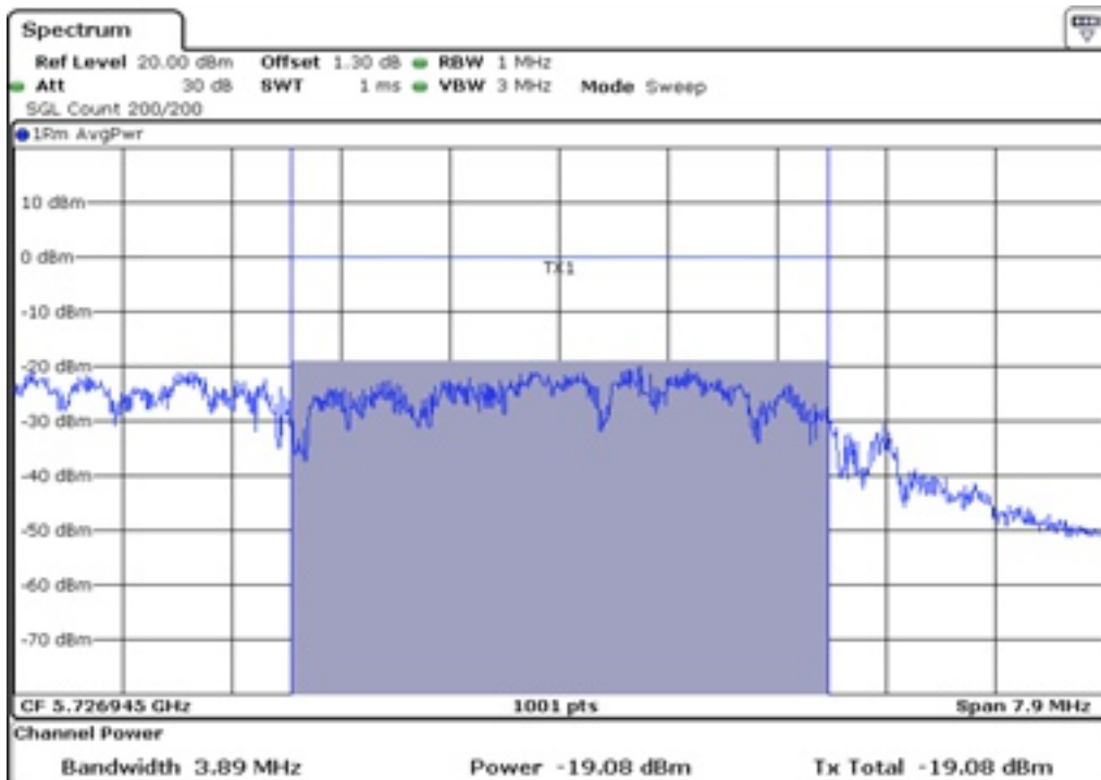
4 Stardle Maximum Conducted Output Power_UNII2C
