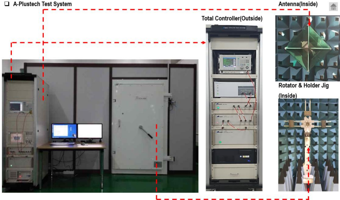
CTIA OTA (Over The Air)TEST 3D Anechoic Chamber (4 × 2.5 × 2.5 m)
