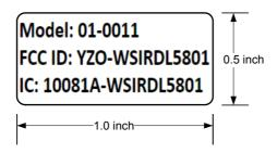
2) Location: To be placed at 'A' or 'B' on the back of the board as marked below or other redline approved location.
