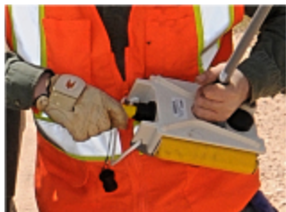
Figure 2–7 Installing the Geophone
