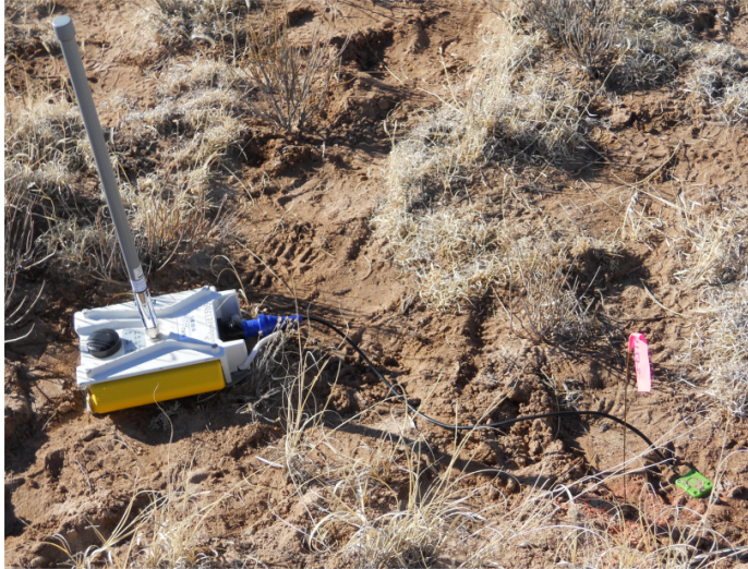
Figure 2–3 WRU with Geophone
