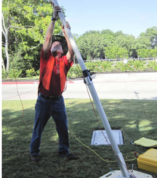
Figure 4–39 Walking the Mast to Vertical 3
