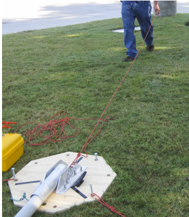
Figure 4–33 Securing Guy Line to Base
