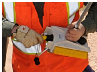
Figure 2–9 Installing the Geophone
