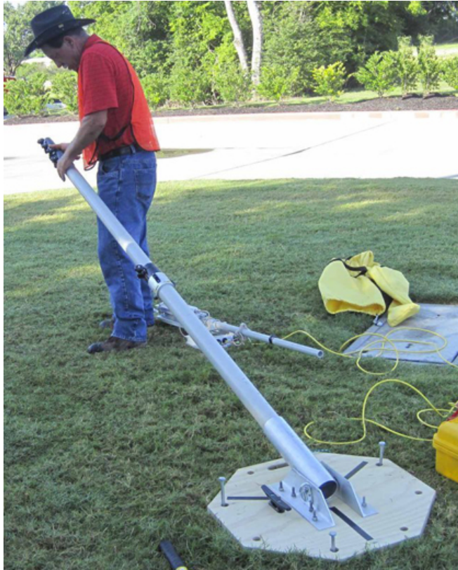
Figure 4–31 Inserting the Mast into the Base and Extending the Mast
