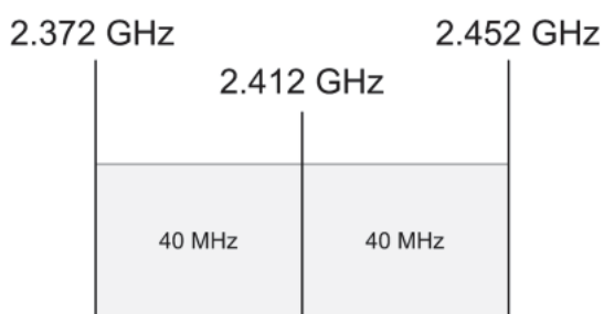
Figure 5–1 Channel, 80 MHz Wide Frequency Band
