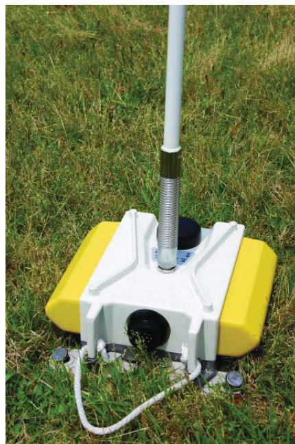
Figure 2–19 WRU Anchored with Anchor Plate
