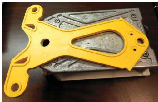
Figure 2–14 Anchor Plate and WRU Alignment
