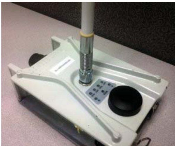
Figure 2-9 Antenna with Spring Relief
