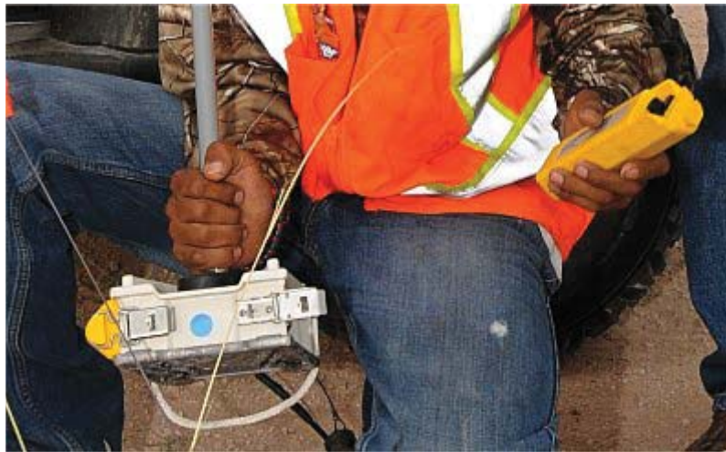
Figure 2–6 Installing the Battery
