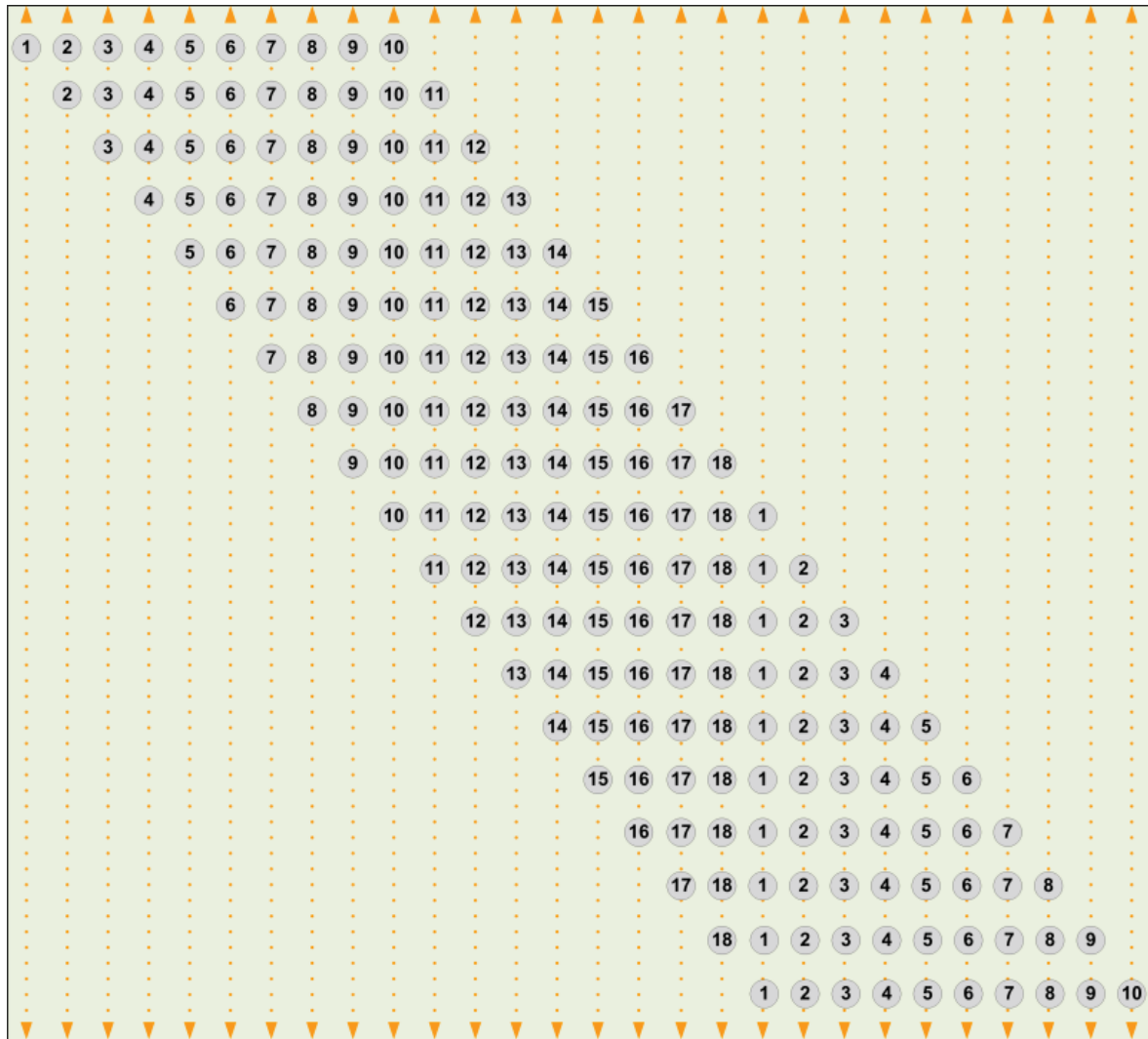
Figure 4–24 Rolling Scheme, 18 Pole Backhaul, 10 Poles in Use
