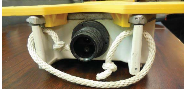
Figure 2-15 Anchor Plate at WRU Geophone End
