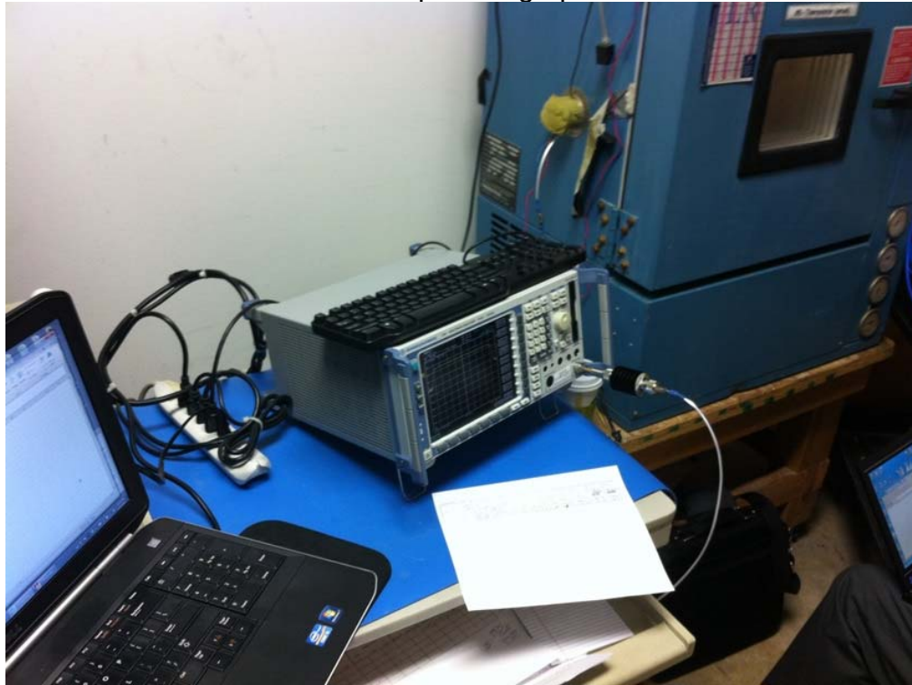
RF Conducted Test Setup; Connected Equipment*
