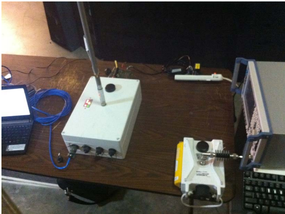
RF Conducted Test Setup; Connected Equipment with LIU* (LIU on left couples commands to EUT by radiated means.)
