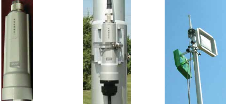
Figure 3–8 Line Radio and Antennas, Bullet
