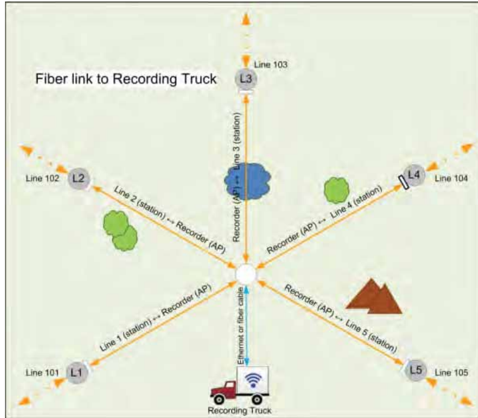
Figure 5–26 Connecting the Recording Truck with Fiber
