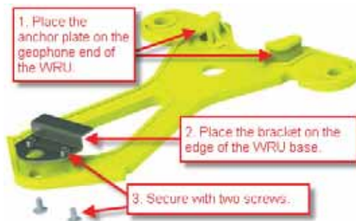
Figure 2–13 Attaching the Anchor Plate to the WRU
