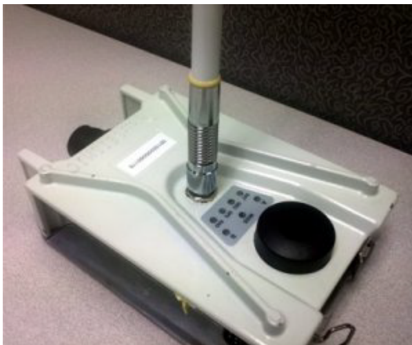
Figure 2-9 Antenna with Spring Relief
