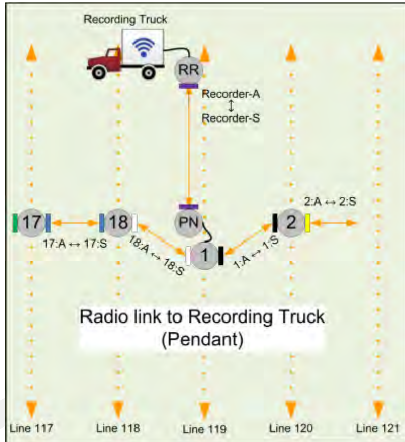
Figure 4–27 Connecting the Recording Truck with a Pendant Radio Link
