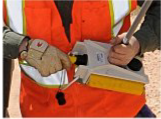
Figure 2–7 Installing the Geophone
