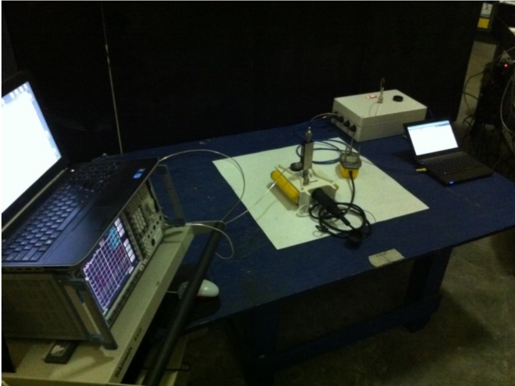
Figure 1: RF Conducted Test Setup
