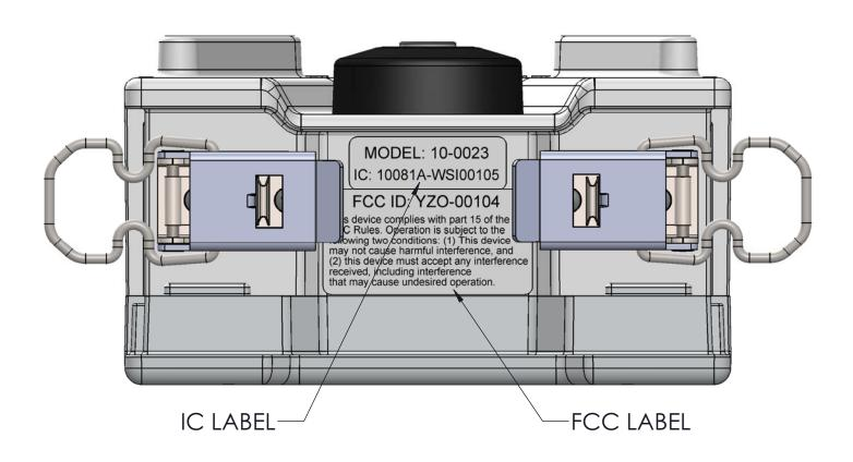
Wireless Seismic, Inc. WRU Model 10-0023 Label Location Diagram
