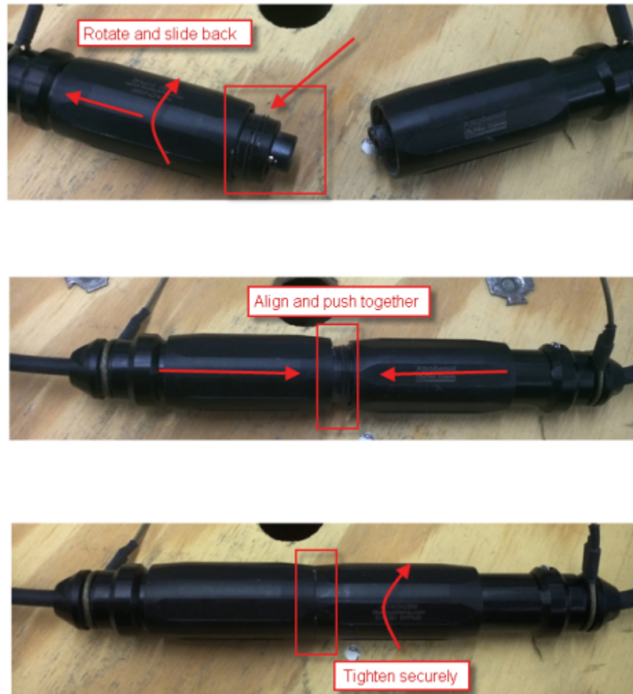
Figure 6–1 Fiber Optic Cable Connector
