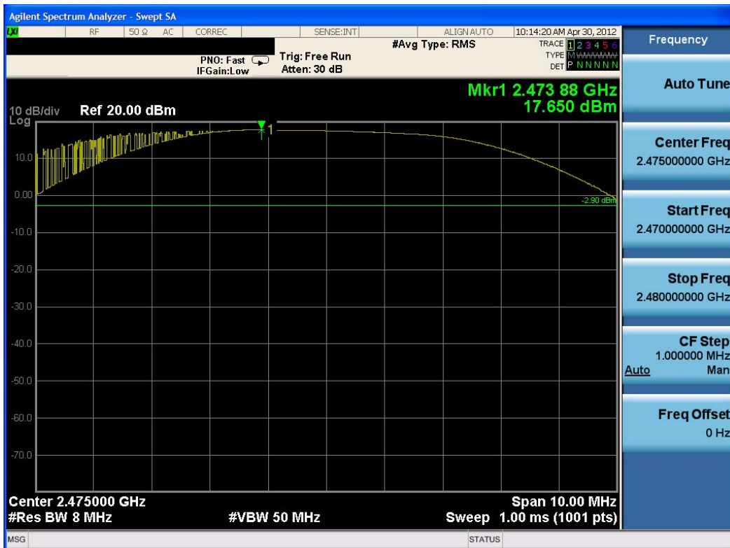
Plot 6-6. Conducted Power (High Channel)
