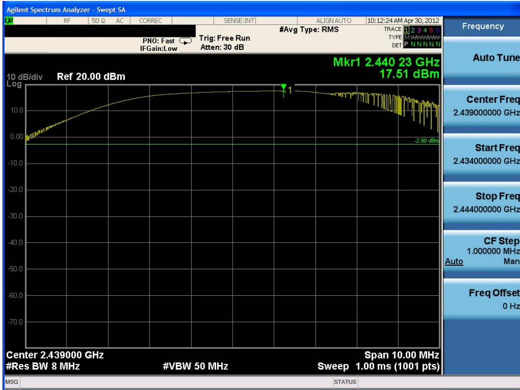
Plot 6-5. Conducted Power (Mid Channel)
