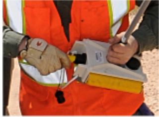
Figure 2–15 Installing the Geophone
